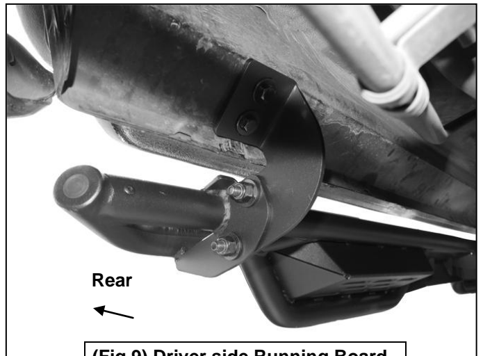
(Fig 9) Driver side Running Board attached to rear Bracket
