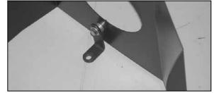
9. Install the small heat shield mounting bracket (070812) with the provided spacer onto the heat shield as shown.
