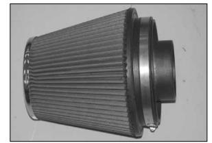
27. Install the radius filter adapter into the K&N $^{\odot}$  air filter and secure with the provided hardware as shown.
