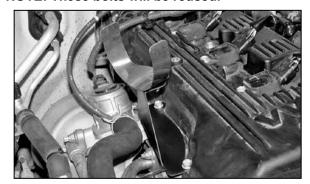
15. Install the tube mounting bracket assembly onto the valve cover using the factory bolts removed in step #14.
