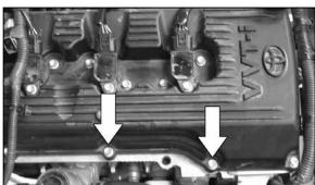
14. Remove the two valve cover bolts shown. **NOTE: These bolts will be reused.**
