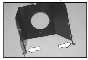
8. Install the two heat shield brackets (07159) onto the heat shield as shown with the provided
