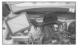
5. Unlatch the air box retaining clips, disconnect the fuel pressure regulator and crank case vent hoses, then lift the intake tract off of the throttle body as shown.
