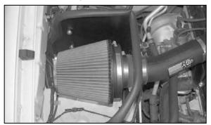
29. Install the K&N® air filter onto the intake tube as shown.
