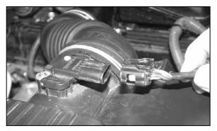
2. Disconnect the mass air sensor electrical connection and unclip the three wire harness retaining clips from the intake tract.
