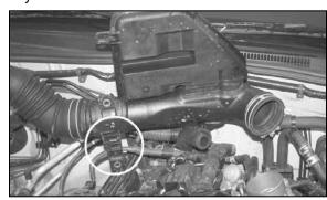
6. Disconnect the wire harness retaining bolts shown and then remove the lower air box from the vehicle.
