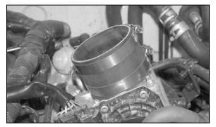
16. Install the provided silicone hose (08756) onto the throttle body and secure with the provided hose clamp.
