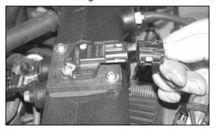
31. Reconnect the mass air sensor electrical connection as shown.
