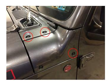
**Step 3:**Locate and remove the factory hardware. \*\*Note: The hardware will not be reused.
