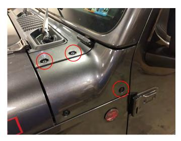
**Step 3:** Locate and remove the factory hardware. \*\*Note: The hardware will not be reused.
