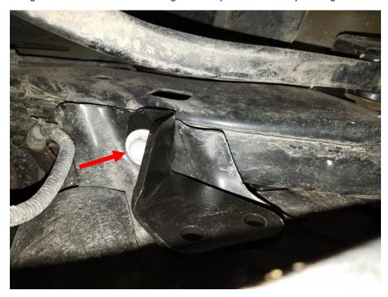
**14.** Insert the supplied nut plate as shown behind the rear corner mounting location.
