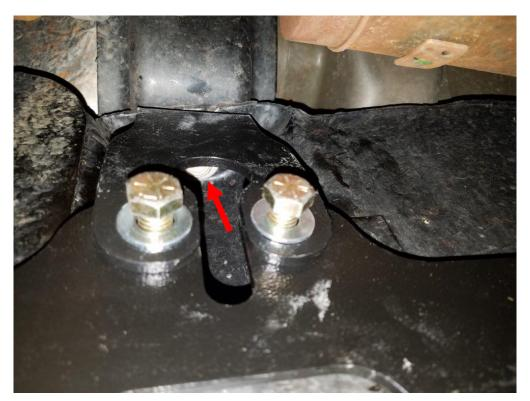
7. Repeat step 6 on the inner on the inner side of the gas tank at the middle mounting location. Then use an 18mm socket with extension to tighten all 5 stock 18mm bolts that you removed. Torque to 73 ft/lbs.
