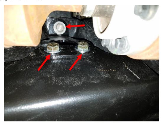
12. Remove the 18mm bolt on the outer rear corner of the gas tank. It is located behind the right rear tire.
