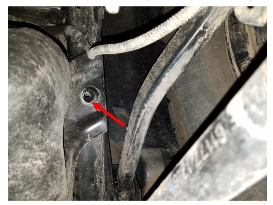
13. Install the angled bracket as shown below using the factory 18mm bolt. Only hand tighten 1-2 turns for now.
