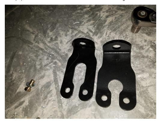
6. Using the correct bracket described in step 5, attach the inner side of the skid plate. Install the stock bolt removed in step 3, using an 18mm socket and socket extension. For now you only want to hand tighten the bolt about 1-2 turns. Then install the supplied bolts and washers as shown below. Tighten to 60ft/lbs using a 16mm socket.
