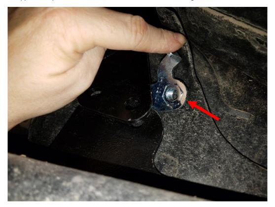
**15.** Use the tab on the nut plate, position the plate and hand tighten the supplied bolts and washers. Then using a 16mm socket, tighten to 60ft/lbs.
