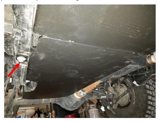
**10.** Using an 18mm socket, remove the inner rear mounting bolt shown below. Then install the mounting bracket as shown below. At this point only hand tighten the 18mm bolt about 1-2 turns. *Note: Notice this bracket is slightly different than the other 2 inner brackets.*
