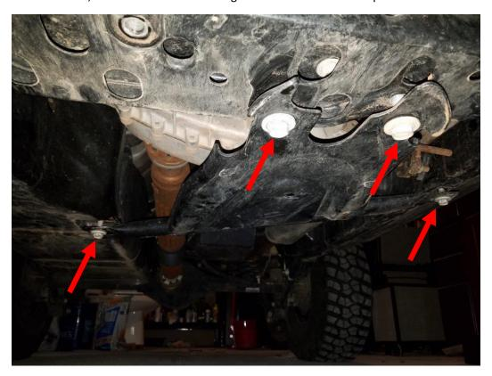
2. Using an 18mm socket, remove the 3 bolts holding on the factory gas tank skid.
