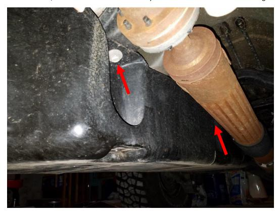
**4.** Now lift into place the front half of your new skid plate. To do this, you can use a floor jack to lift it into place and hold it. Then insert and hand tighten the 3 factory bolts shown below.
