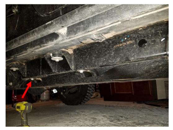
**9.** Now lift the rear half of the skid plate into place, and hand tighten the 18mm bolt removed in step 8. You will need to lift the inner side of the skid plate into place then the outer side. At this point the skid plate should be held up on the inner side by the attached mounting bolts.
