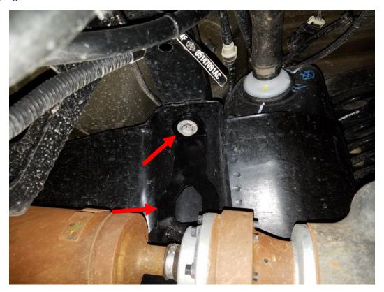
**11.** Install the supplied bolts and washers as done in step 6. Using a 16mm socket, tighten to 60ft/lbs. Then you can mostly tighten the 18mm bolt.
