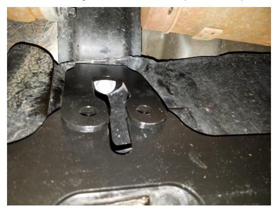
8. Use an 18mm socket to remove the 18mm bolt shown below.
