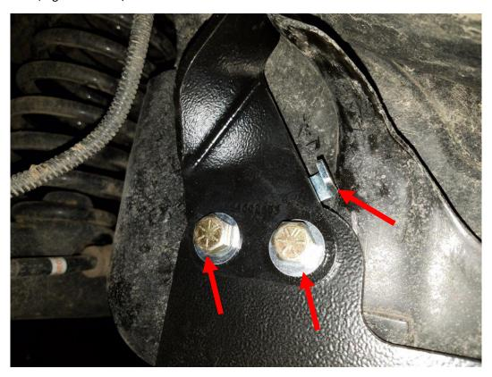
**16.** Using an 18mm socket, tighten the factory bolts from steps 9, 11, and 12 to 73ft/lbs.
