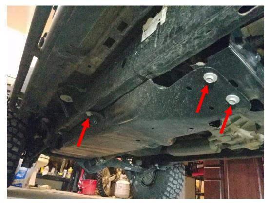
**3.** Using an 18mm socket, remove the 2 bolts shown. They are located on the inner side of the gas tank.
