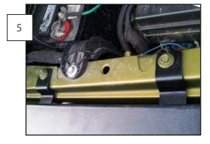
Open the hood and remove the (2) top fender bolts. Move the snorkel into place and reinstall the bolts through the snorkel brackets and into the fender. Make sure the snorkel is inserted into the factory air box intake.
