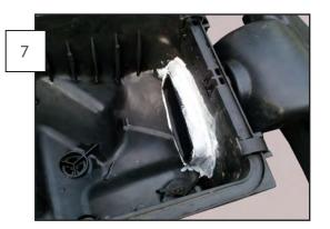
Seal the snorkel to the factory intake with waterproof caulking. Allow the caulk to cure before driving. Seal both the inside and outside of the box. Also coat the bare metal along the cut edge of the hood to prevent rusting.
