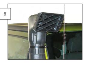
Place the snorkel intake on top of the snorkel tube. Secure it with the supplied pipe clamp.
