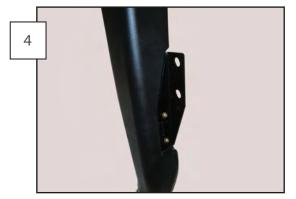
Install the supplied upper bracket to the snorkel using the supplied allen head bolts.
