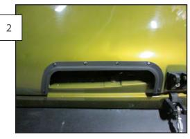
Place the hood bezel around the hole that was cut out. Drill (7) 1/8" holes, at each rivet spot. Install the supplied rivets through the holes and secure them with a rivet gun.
