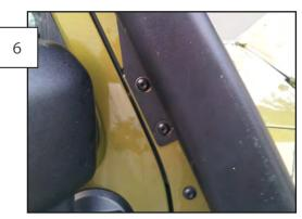
Remove the 2 upper T40 Torx bolts from the passenger side of the windshield frame. Hold the snorkel in place and reinstall the 2 T40 Torx bolts through the upper bracket and into the passenger side of the windshield frame.
