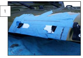
Place the supplied template 23mm back from the passenger hood latch. Tape the template to your hood and protect the rest of the vehicle from scratches and nicks. Using a 1-3/4" hole saw drill two holes where the template shows and connect them with a rotarty cutter.
