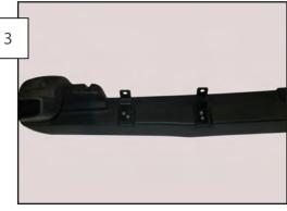
Install the supplied lower brackets to the snorkel using the supplied allen head bolts and washers.
