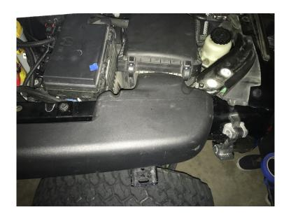
2. Find middle point of template with tape measure, drop hood and measure air intake by lining up center point of template and center point of air intake section on snorkel. Once aligned attach template to bottom lip of hood with painters tape.
