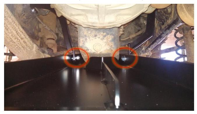
4. Attach the middle hole on the skid plate to the transmission cross member with the 12mm bolt. DO NOT USE ANY OTHER BOLT. This bolt gets threaded into a welded nut. Install the 1/2" bolt on the left with a matching nut.
