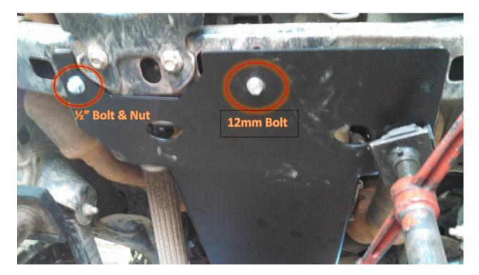
5. Drill out the last hole, on the right side, to fit the last 1/2" bolt.
