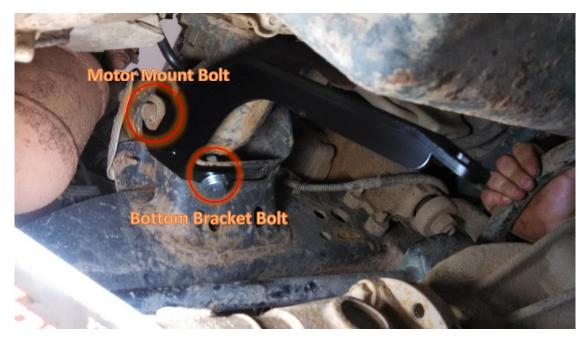
2. Install the passenger side bracket. Repeat STEP 1 on passenger side.
