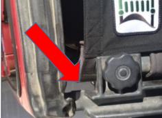
2. Feed the strap into the metal teeth on the opposing side. Be sure that you feed the straps into the teeth like in the picture below
