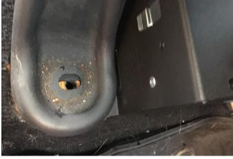
• Reinstall the anchor bolts removed in step 5.
