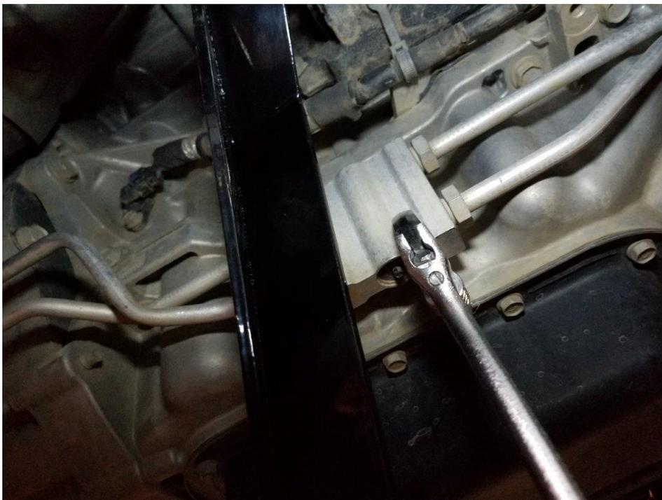
7. If equipped, you will need to remove the bar just in front of the mid vehicle cross member. Use an 18mm deep well socket to remove the 3 bolts as shown. Keep the center bolt, you will need it for the skit plate.
