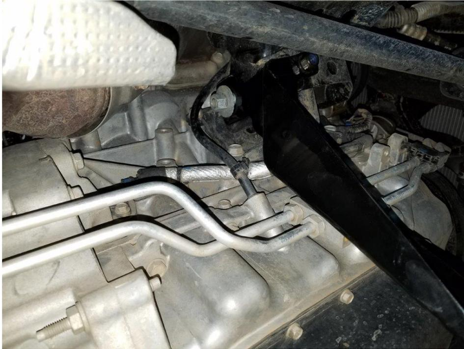
6. (For Automatics only) If the transmission cooling lines come in contact with the bracket you will need to make a minor adjustment to the cooling lines. Using a crescent wrench on the expansion block, carefully bend it toward the engine until it is clear of the bracket.
