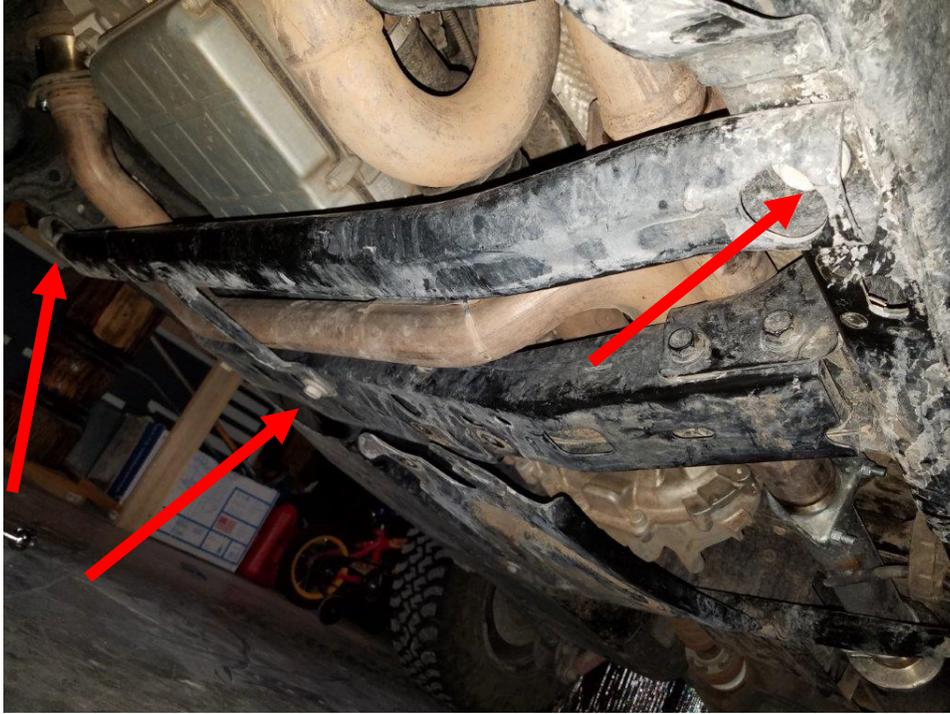
8. If equipped with the stock transfer case skid plate you will need to remove the front 2 bolts and loosen the rear 2 bolts. This transfer case plate will bolt over the Rugged Ridge Engine skid plate. Note: If you have the rugged ridge transfer skid plate, the engine skid plate will bolt over it.
