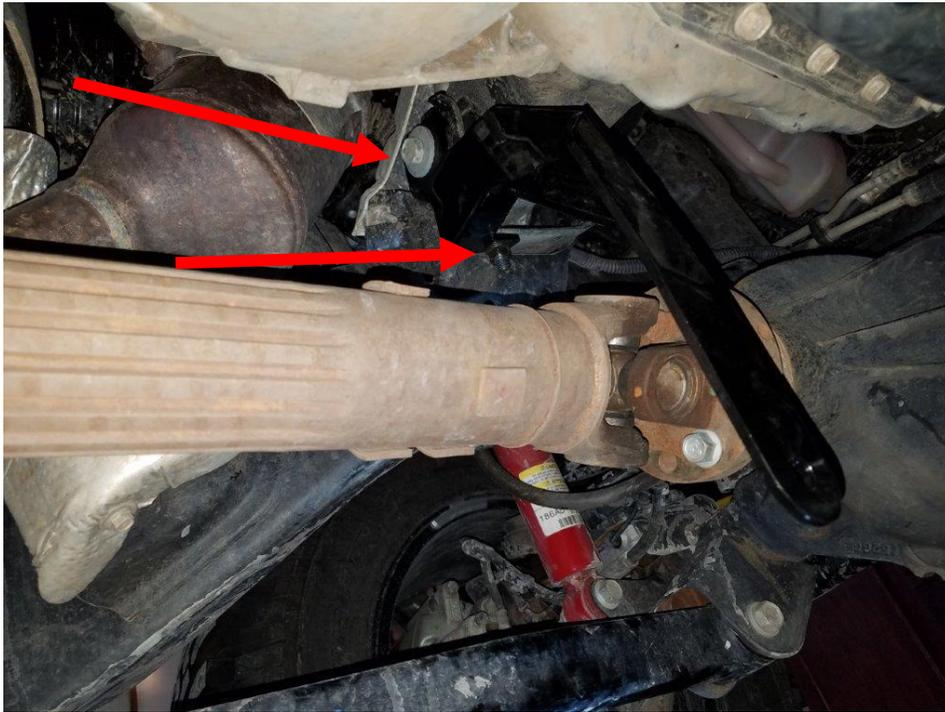
4. Now use an 18mm socket to loosen the passenger side motor mount nut. Loosen the nut as shown below but leave the nut on. Then install another supplied bolt and washer in the rear hole of the passenger side motor mount bracket as shown. *Note: For me the bolt would not fit in the hole, so I had to shorten the bolt. If yours is the same way you will need to use a dremel to trim about 1/4" off the end of the supplied bolt.*
