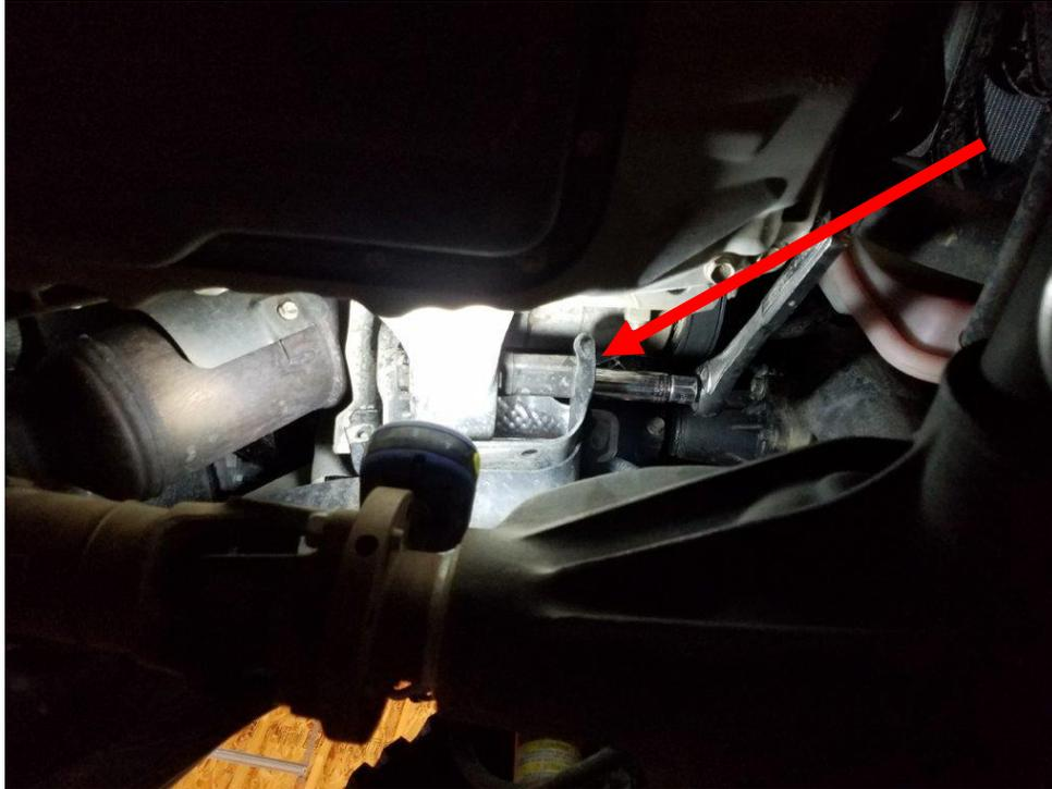
2. When you tap the bolt to the rear it should give you room for the bracket as shown below. Then insert one of the supplied bolts with a washer into the rear hole on the bottom of the motor mount bracket as shown below.
