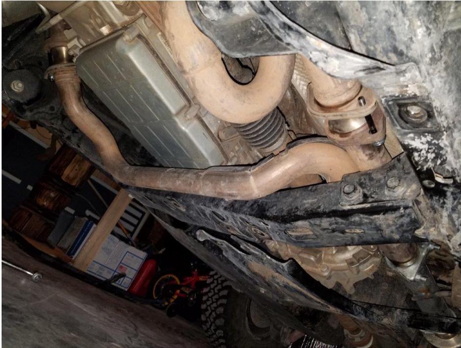
10. The bolt holes do not completely line up so you will need to drill a new hole for the center cross member bolt. I recommend installing the plate with the 2 outer bolts so you can mark the location of the center bolt. The arrow below shows the new hole you will need to drill. Use a drill with a 1/2" drill bit.
