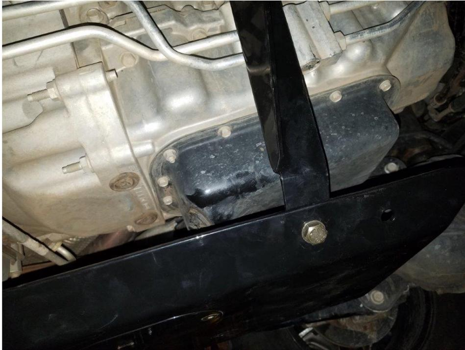
**14.** Once all of the bolts are installed and lightly tightened you can completely tighten all of them. Torque the motor mount bolts to 45ft/lbs, the 3 cross member bolts to 65ft/lbs, and the transfer case skid plate bolts to 65ft/lbs.
