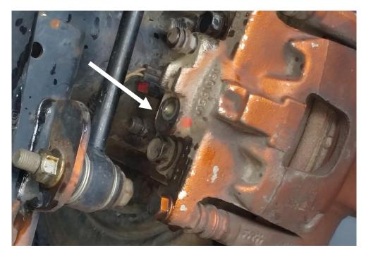
**4.** Add the new copper crush washers (provided in kit) onto either side of the brake hose connector. Using the 15mm socket, carefully reattach the bottom end of the brake line to the caliber with the banjo bolt and tighten.
