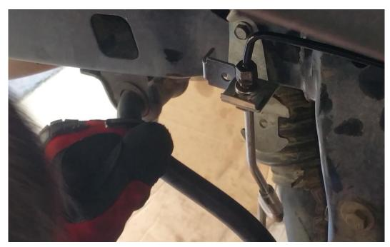
**3.** Using the 15mm socket, remove the banjo bolt from the caliper.
