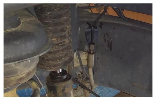
2. Use the 12 mm flare nut wrench to disconnect the brake line fitting.
