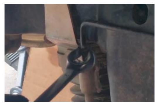
**2.** Using an 11mm socket and wrench, remove the bracket from the frame.
