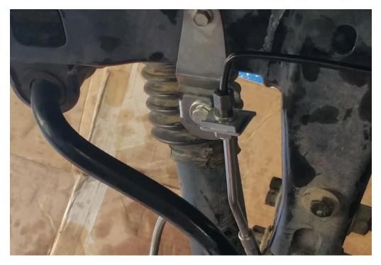
6. Bleed all four brake lines before reinstalling the wheels.
