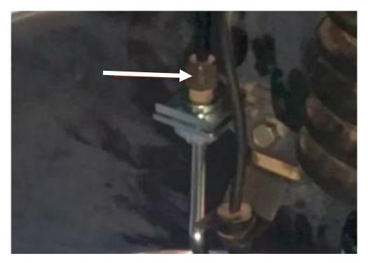
**9.** Add the new copper crush washers (provided in kit) onto either side of the brake line connector. Using the 15mm socket, carefully reattach the bottom end of the brake line to the caliber with the banjo bolt and tighten.
