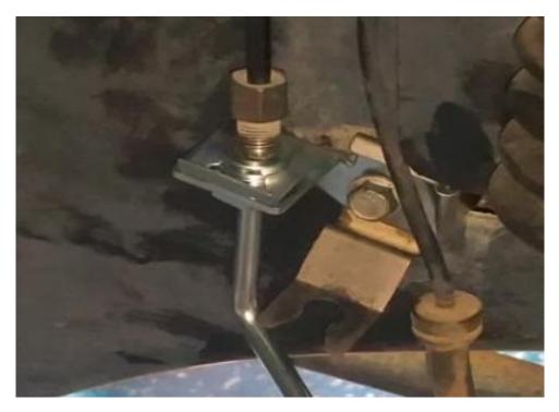
7. Slide the wheel speed sensor cable into the bracket
