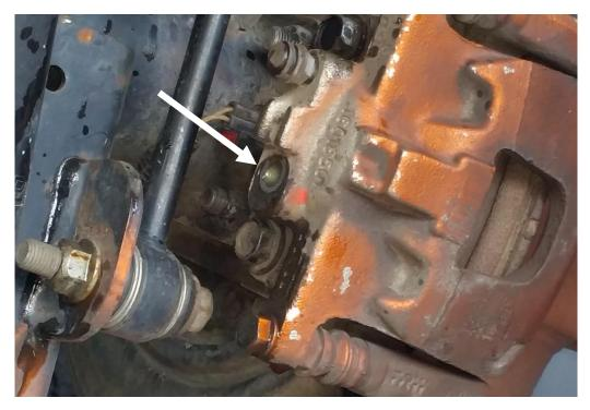
**5.** The new brake line bracket and the stock bracket that holds the speed sensor to the frame may not match up. You may need to trim the tab off of the speed sensor bracket.
