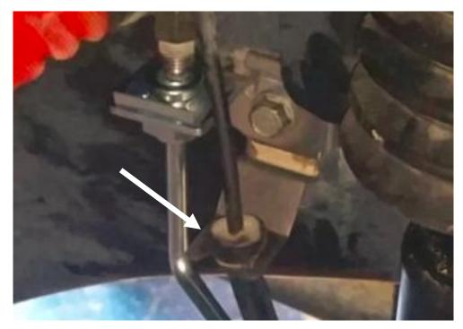
**8.** Using the 12mm flare nut wrench, reconnect the top of the brake line to the bracket. Do not over tighten.
