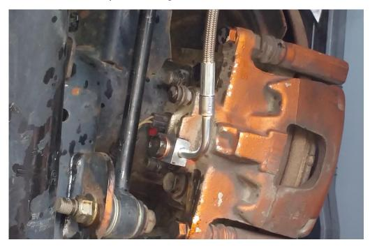
5. Using an 11mm socket and wrench, connect the bracket to the frame. Using the 12mm flare nut wrench, reconnect the top of the brake line to the bracket. Do not over tighten.
