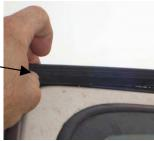
**Step (3):** Push the front support bow all the way forward. Bow must slip into notch in the belt rail.
