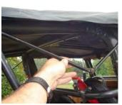
Step (4): Release the rear corners of the top. Pull gently down and then out to release the plastic strip from the retainer on the vehicle.
