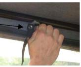
**Step (3):** Pull down on spreader bars and push rear support bow forward.
