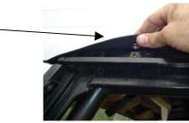
Step (12): Unfasten the plastic retainer at the bottom of the fabric door and remove it from the vehicle. User a razor knife to cut the stitches on the old door covers and remove them from the door frames.
