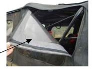
Step (1): Remove the quarter windows and rear window. Remove the metal tailgate bar from the bottom of the rear window and set to the side. It will be reused.
