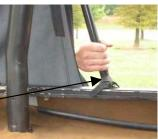
**Step (4):** Insert rear corners of top into rear corner retainer rails.
