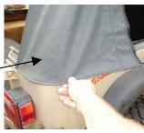
**Step (5):** Pull the bottom rear support bow back until it snaps into the notch in the side rail.
