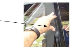
Step (8): Slide the plastic strip on the bottom of the side curtain into the side retainer. Start at one end of the strip and work along to the other end. Close the top and rear zippers on the side curtains
