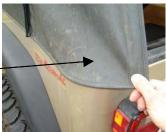
**Step (5):** Unsnap the old top from above doors, remove front plastic strip from windshield channel and remove old top.
