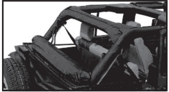
Step 1: Remove plastic door surrounds if equipped. Gently pull down on front molding near windshield. This will allow old cover to be removed and the new cover placed under trim (pic.1).
