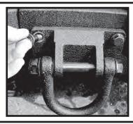
Step 2. Align the new D-Ring with the holes in the XHD bumper and fasten using the existing hardware.
