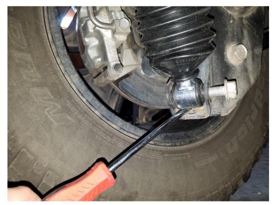
9. Use a torque wrench to tighten the lower shock bolt to 65ft/lbs. Then torque the top shock bolts to 37ft/lbs.
