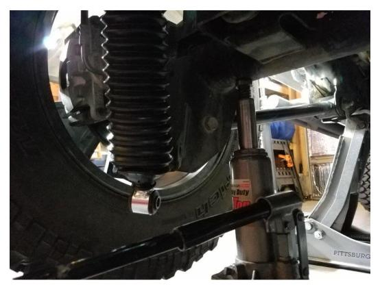
7. Even with the axle lowered completely, the shock may not fully line up. You can push up on the shock to compress it slightly then put it in the lower mount.
