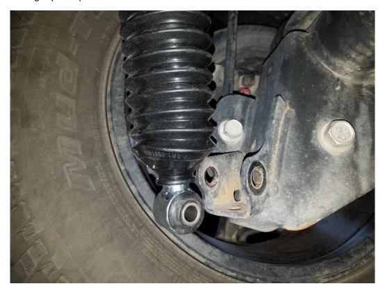
8. Use a flathead screwdriver to pry the shock up enough to insert the lower bolt.
