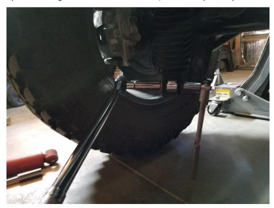
10. Before driving with the new shocks, you will need to make sure you have the right amount of bump stop to keep from bottoming out the shocks. Lower the Jeep back to the floor. Now measure how much more down travel you have before bottoming out the shock. Feel through the boot for the point where the shock tube ends, and feel where the lower shock mount starts. Measure between those 2 points. Mine measured 4 ½"
