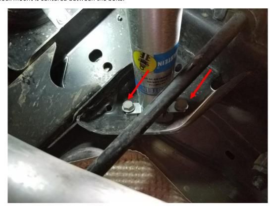
6. Then lower the jack holding up the axle. Lower it until the lower shock mount lines up with the bottom of the shock.
