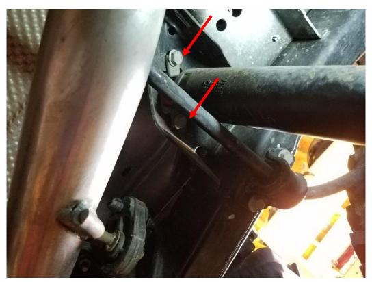
5. Put the new shock in place on the and snug the upper shock bolts, but do not completely tighten yet. Make sure the shock mount is centered between the bolts.
