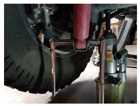
4. Use a 16mm socket with extension to loosen the top shock mount bolts. Remove 1 bolt completely, and just loosen the other. Then you can remove the shock.
