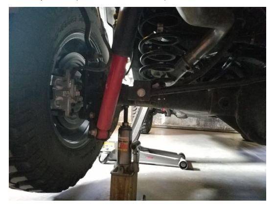
3. Using two 18mm sockets, remove the lower shock bolt.
