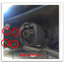
2. Unscrew the fog lights from the factory bumper and reinstall them on the new bumper using the provided sheet metal screws. See below.
