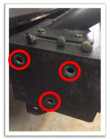
3. Attach stubby ends to the bumper using M12 hardware. Bolt heads should be inside stubby ends and lock nuts inside center section.
