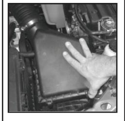
**44** - Disconnect air tube from air box and intake. place to the side. Sensor wire may need to be disconnected. (3.6L shown)
