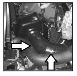
74 - Reinstall windshield bracket removed in step (2). Start and tighten the upper side M12 bolts and front M12 bolts as shown .
