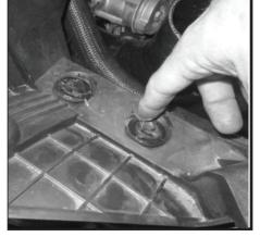
**68** - Insert (2) M8 x 35 bolts with (2) M8 flat washers through lower air box mounting holes and rubber grommets. Apply a small amount of sealant to washers.
