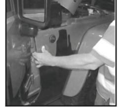
**104** - Secure top of fender to inner fender frame. Battery tray support will need to be lifted to allow fender to slide under support.
