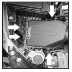
**96** - Reinstall air filter removed in step (41). It is recommended that a high flow air filter be used. Either a washable (oil free) design like Rugged Ridge P/N: 17752.05 or K&N oil type can be used.
