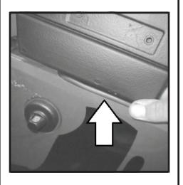
**38**- Apply a very small amount of super glue to inner corners of fender gasket. It will be easier to start at on end and work around opening. Applying glue as needed. This will insure gasket remains in place during reasembly.
