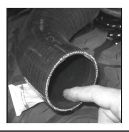
**63** - Apply a thin film of sealant around end of aluminum air tube. An excessive amount may cause the elbow to slide off air tube when tightened.
