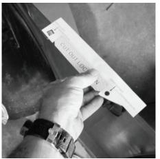
24- Enlarge the (4) 1/8" guide holes with a 5/16" bit. Carefully open guide holes making sure to place wood block over holes. Drill bits can grab thin sheet metal and shoot forward damaging fender. Increase hole size if needed.
