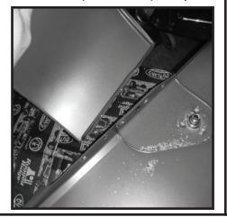
23- Using a small drill bit (1/8" is recommended) drill center guide holes into each spot weld as shown. A wood block should be placed inside of cowl as guide holes are drilled. This will reduce the chance of damage to cowl sheet metal.
