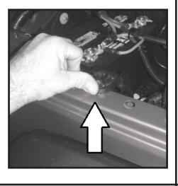
**19** - Reach under plastic fender and disconnect side marker light. Socket can be removed by turning socket counter clockwise and pulling away from fender.
