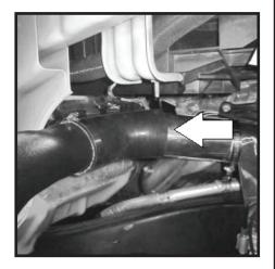
77 - Apply a thin bead of sealant around the lower section of the snorkel main body. Spread sealant evenly around the outside of the outlet. Do not use excessive amount of sealant. A thin layer will insure a tight seal.
