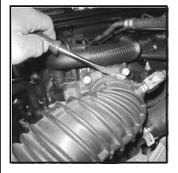
**45** - Disconnect factory air intake tube from upper air box, place to the side. Upper air box will be reused. Do Not Discard.
