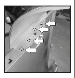
25- With spot welds cleared carefully remove upper cowl from fender. NOTE: Fender can be damaged if welds have not been opened completely.
