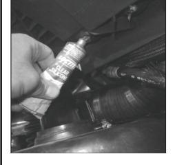
**69** - Install (2) M8 nuts and (2) M8 flat washers to the underside of inner fender mounting plate. Add sealant if needed to insure a water tight seal.
