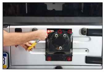
STEP 1 // Remove the rear tire and the (5) 13mm bolts securing the tire carrier.
