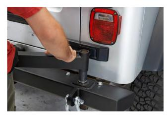
**STEP 10 //** Install the swing arm by sliding it over the post on the bumper. \*\*Note: Bumper post and swing arm must be greased liberally to prevent corrosion.
