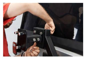
**STEP 13** // Finally, install the rear tire carrier onto the rear swing arm using the (4) 18mm bolts and nuts and tighten them down. Then, reinstall the rear tire. Installation is now complete.
