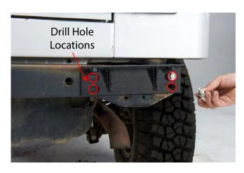
STEP 6 // Using the supplied brackets and 18mm hardware, mount them to the vehicle in the factory mounting holes as pictured. \*\*Note: The (2) inner mounting holes locations will need to be drilled. Drill using a 3/8" drill bit & drill.
