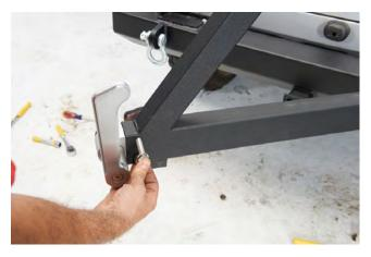
**STEP 12** // Slide the latch assembly into the swing arm and secure using the 17mm bolts and nuts.
