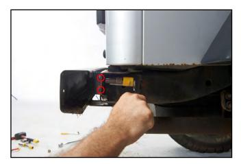
STEP 4 // Using an 18mm socket, remove the (4) bolts securing the rear bumper.
