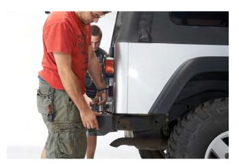
**STEP 7** // Slide the new bumper into position on the mounting brackets and line the 4 holes on the top of the bumper up with the 4 holes on the mounting plates.
