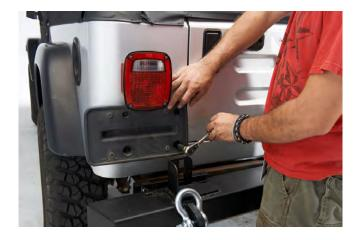
**STEP 8** // You may have to remove the plate bracket for extra clearance. Using a 10mm socket, remove the plate holder.
