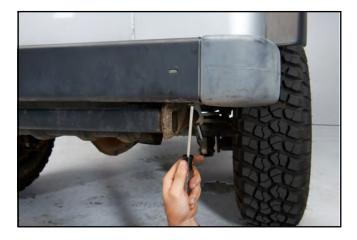
STEP 2 // Remove the Torx screws, on the top and bottom, holding the end caps on the rear bumper. Remove the end caps.
