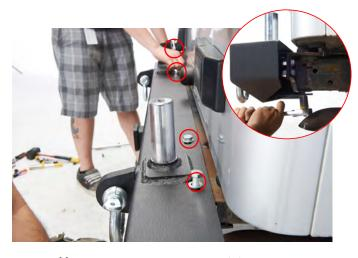
**STEP 9** // Using the 18mm supplied (6) bolts, washers and nuts, install the rear bumper onto the vehicle, leaving it loose for adjustment. Once it is in place and centered, tighten all the bolts.
