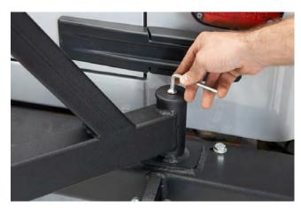
**STEP 11** // Install the top cap and secure it using the M10 allen bolt.
