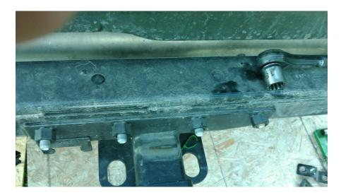
5. Remove the 8 bolts holding the stock tire carrier with your 13 mm wrench. Open your tailgate and carefully pop off the vent using a flathead screwdriver. Unplug the wire connection.
