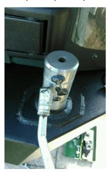
9. Place the tire carrier portion on. Place the black washer and the allen head bolt in to tighten. On the opposite side, install the handle using the two 17 mm bolts. Measure the radius of your tire from one nut hole to the edge of your tire. On the tire carrier, measure from the center stud to bumper where your tire will sit, to ensure your tire will not hit the bumper. This will give you a good idea of where to place your tire so it does not hit your bumper when you shut the gate.
