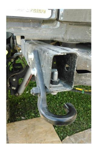
4. Remove the 4 bolts for the receiver if necessary. Take the new mounting bracket and slide behind the remaining beam. Line your long bolts halfway through for now.
