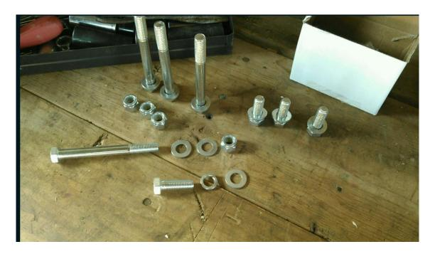
2. Remove the existing bolts holding the current bumper on, two on each side, with your 15 mm wrench.
