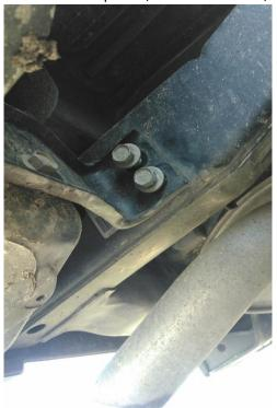
3. Remove the bolts to remove the tow hook if needed
