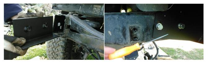
7. Next, go underneath the Jeep and push the bolts through. Tighten the nuts on the opposite side, followed by completely tightening the short bolts on the side. This will complete the bumper portion of the install.
