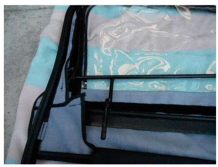
6. Force the front lower corner into the door skin being careful not to snag or damage the skin, do not secure Velcro yet.
