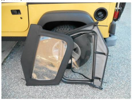
2. Using a box cutter or razor work along the seams to remove factory door skin from factory frame
