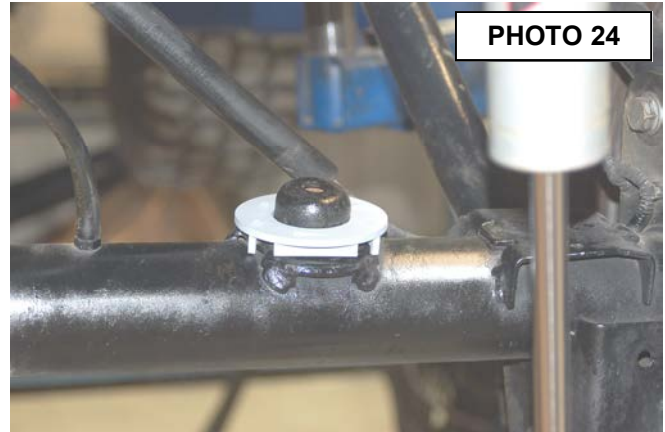
Install the lower control arms
