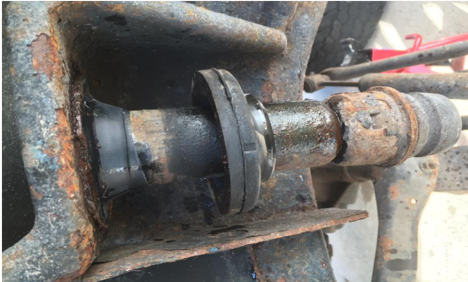
From left to right, stock coil spring isolator, bump stop cup, rubber bump stop
