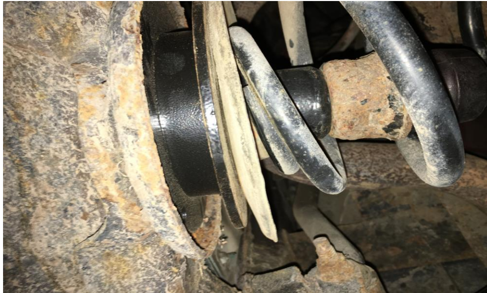
From left to right, New spacer, coil spring isolator, bump stop cup and bump stop.
