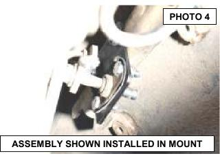
Due to factory variations on the shifter rod bracket, it may be necessary to modify the shifter bracket by slightly bending the mount on the rod to clear the shifter bracket or shifter bracket bolts. After noting how much to bend the bracket to clear, remove the shifter assembly and bend the bracket as shown to slightly clear the bracket / bolts. Do not over-bend!! See Photo 13.
