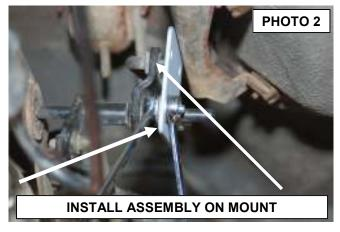
4. Install the supplied drop bracket on the stock tunnel bracket with the supplied 1/4" x 3/4" bolts/washers & nuts. Tighten hardware using a 7/16" wrench. Check clearance on bolts. **See Photo 3 & 4.** In Photo 3, bracket is shown removed to show mouting location. It is not necessary to remove the bracket although it can be removed to ease installation.
