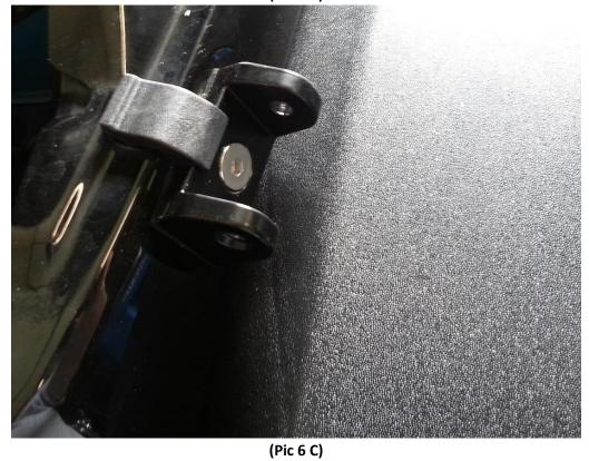
6. Place lower latch portion of the Rugged Ridge Aluminum Hood Catch Kit back into the base. Use the (2) 5 MM Allen wrenches to tighten the swivel bolts back into place. (Pic 7)
