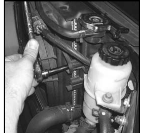
Remove upper shroud bolt
