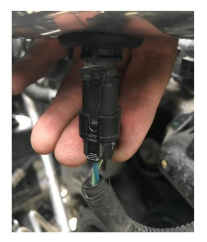
19. Once the O2 sensor is connected, the next step is to reattach the rubber intake tube to the fan shroud. Use the provided attaching clamps.
