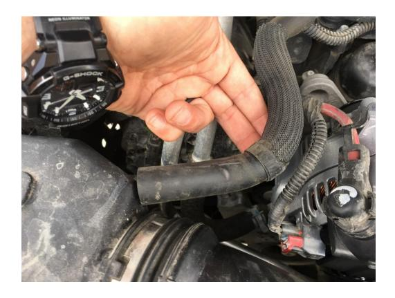
4. After I had the O2 plug and the PVC hose off, the next thing to disconnect is the take the bolts holding the intake tube to the fan shroud. This is done with the 12mm socket and wrench.
