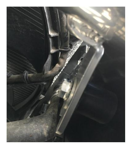
17. Using the (2) provided hose clamps, attach the PVC tubing to the new intake tube.
