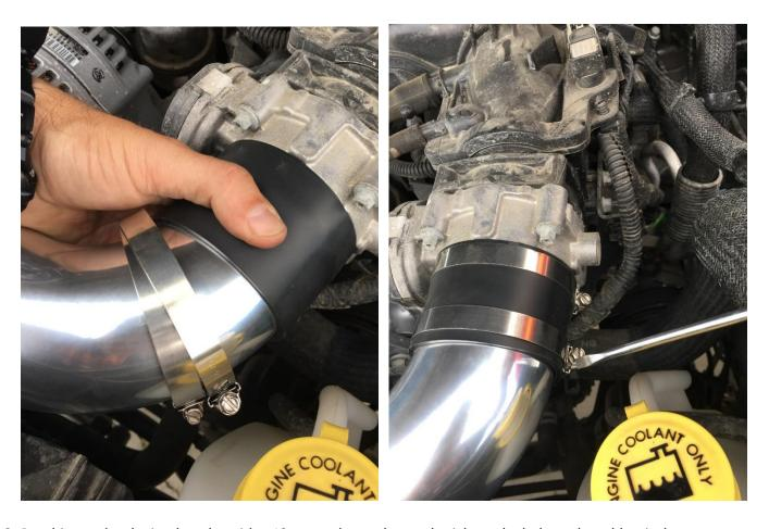
16. Reaching under the intake tube with a 12mm socket and wrench, tighten the bolt on the rubber isolator.
