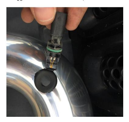
14. After the O2 sensor is installed, grab the rubber isolator and bolt it on, using the provided hardware. You will use the 13mm socket for this.
