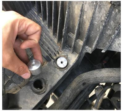
10. Now grab the heat shield out of the box, and take the two M6 mounting bolts, two washers, and M6 nuts and feed them through the holes in the heat shield. Once the bolts are in the heat shield, simply insert the bolts into the aluminum spacers and attach the washer and M6 nut from underneath the heat shield using the 12mm socket. Then reattach the fan shroud screw through the hole on top of the heat shield using the 10mm socket.
