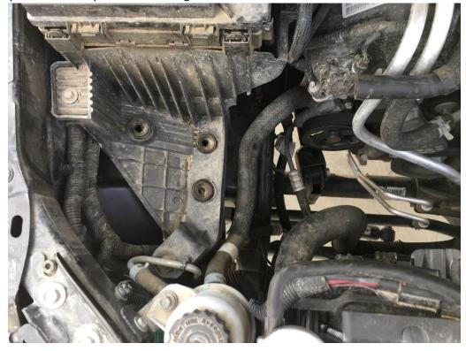
8. Next take the top left fan shroud screw out using a 10mm socket and wrench.
