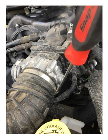
6. Once these steps have been taken open the air box, and lift the entire factory intake tube out of your Jeep.
