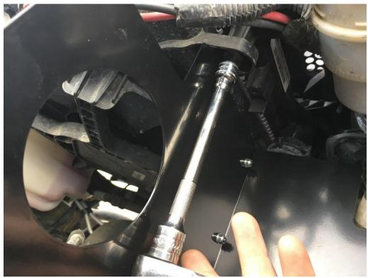
11. Once you have the heat shield installed, attach the provided rubber gasket to both the top of the heat shield, as well as the hole for the intake tube, and cut to the proper length using the tin snips.
