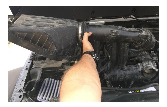
7. Once you have the intake tube out of your Jeep, grab the air box, and pull up sharply. It will pop out of its seat, and then you will be ready to start installing.
