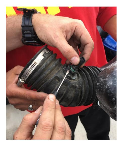
13. Next insert the provided O-ring grommet into the new intake tube, and insert the O2 sensor.
