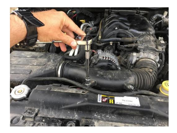
5. Next loosen the hose clamp holding the intake tube to the throttle body.
