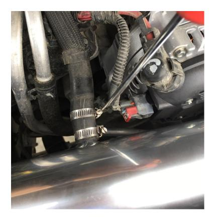
18. Next reattach the O2 sensor plug, it just snaps back on.
