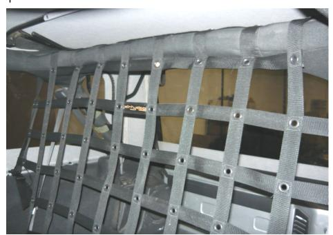
The next step is the straps at the bottom. These are a little tricky. At the bottom of the seat bracket that bolts to the floor. The bracket has two layers of steel with a slot space in between . This is where you need to slide in the webbing. It takes a little wiggling to get it through.
