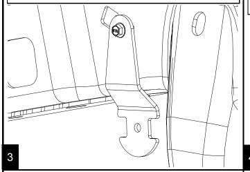
Using a 7/16" wrench and the supplied hardware, bolt the brake line to the bracket with a washer on both sides. Torque bolt to 120 inch-lbs (13 Nm)
