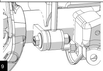
Reinstall the front track bar once the vehicle is sitting on the ground. Torque to 125 ft-lbs. (See 999208 Front Track Bar/Installation)
