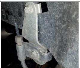
Press the hard brake line against the frame to avoid contact with the sway bar links as the suspension cycles.
