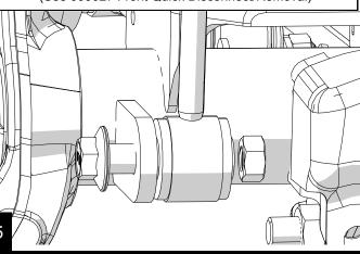
Lower the jack until the spring is free. Remove the coil spring. Be sure to watch the ABS, brake lines and breathers that they are not over stretched..
