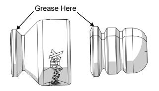
Align the bumpstop, extension and frame cup. Place a block between the frame and the axle bump pad. Raise the axle with a jack until the bumpstop and extension seat.
