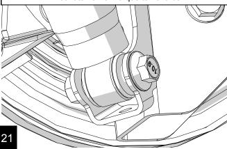
Reinstall wheels and tires, torque to 95-115 ft-lbs. Lower to the ground. Torque all upper control arm bolts to 75 ft-lbs and all lower control arms to 125 ft-lbs.
