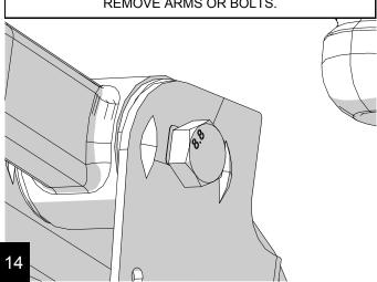
Remove the shock at the axle with an 18mm. (See 999207 Shocks/Rear/Removal)
