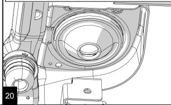
Raise the axle high enough to reinstall the lower shock bolts.
