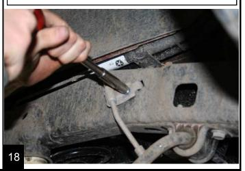
Carefully lower the axle enough to remove the spring. Be sure to watch the ABS, brake lines and breather tubes for overextension. Remove the old spring.
