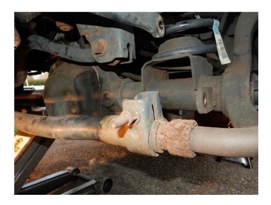
67. Mark the adjuster sleeve of the drag link to note the factory setting, to be used as a base point.
