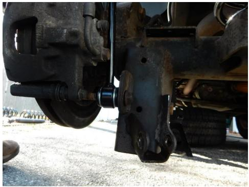
23. Using an 18mm socket and wrench, install provided 1/2"x20 bolt and washer and the 19mm nut and washer to attach the sway bar link to the sway bar on the driver and passenger sides. Torque to 75 ft-lbs.
