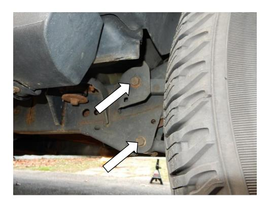
39. Using a 21mm socket, remove the bolt connecting the front track bar to the axle bracket. *Note: A flag nut is used on this bolt.*
