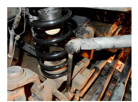
61. Using and 18mm socket and wrench, install the axle side bolt into the sway bar and torque to 75 ft-lbs. *Note: The sway bar link installs to inside of the axle mount.*
