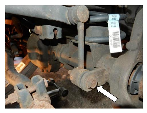
51. Using an 18mm socket and 19mm wrench, remove the upper bolt from the front sway bar links on the driver and passenger sides.
