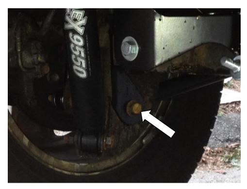
29. Position the provided spacer sleeve between the factory track bar bracket and the axle track bar bracket. Using a 1/2" socket and wrench, install the provided 1/2"x3.5" bracket bolt, washers, and locknut to attach the axle track bar bracket to the factory track bar bracket. Torque to 75 ft-lbs.
