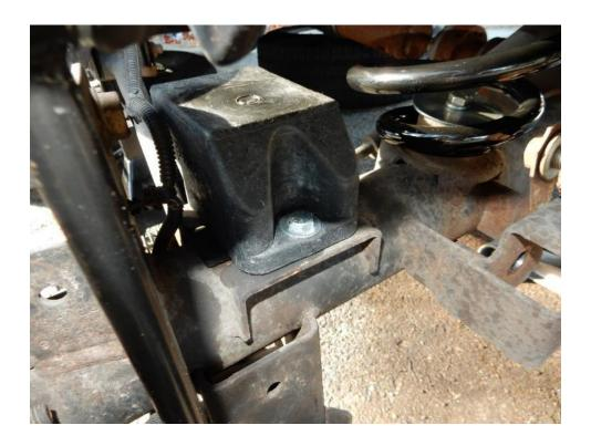
26. Using a 21mm Socket and wrench, remove the lower control arm axle side bolt.
