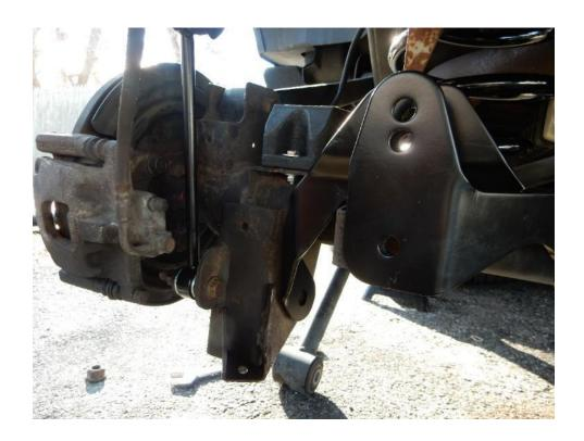
28. Using a 21 mm socket and wrench reinstall the lower control arm bolt. Torque to 125 ft-lbs. *Note: Do not torque bolt until vehicle is on the ground and at ride height.*
