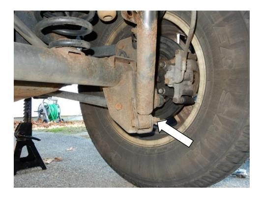
10. Using a 16mm socket, remove upper bolts from rear shocks on the driver and passenger sides, remove the rear shocks.
