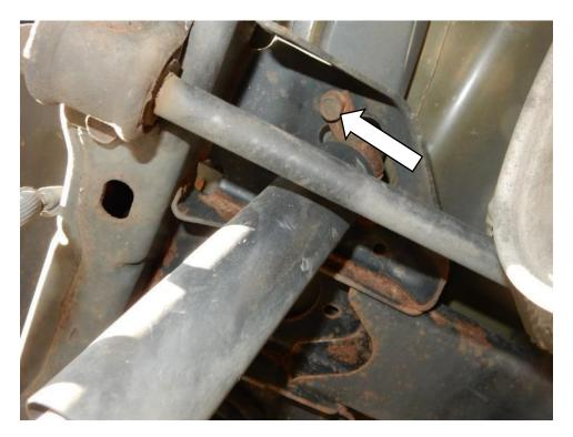
11. Using and 18mm socket and wrench, remove the bolt on the axle side of the rear sway bar links on the driver and passenger sides.
