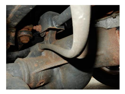
65. Position the front track bar in place at the frame mount. Using a 21mm wrench and socket, reinstall the factory bolt and nut. Torque to 125 ft-lbs.
