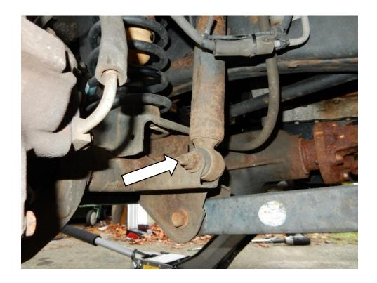
49. Using a 16mm wrench, remove the upper nut from the front shocks on the driver and passenger sides. *Note: a 5/8" wrench can be used just below the shock mount to keep the shock from spinning.*
