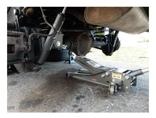
54. Using pliers, carefully remove the factory bumpstops from the driver and passenger sides.
