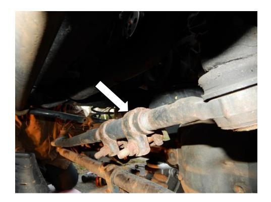
68. Using a 15mm socket, loosen the nuts on the adjuster sleeve of the drag link. Rotate the adjuster sleeve of the drag link clockwise approximately 3/4 of a turn or as needed until the steering wheel is straight.
