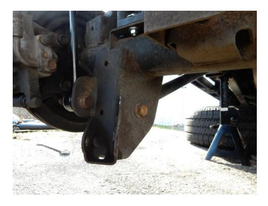
27. Position the rear axle track bar bracket over the factory track bar bracket, aligning the lower control arm bolt holes.
