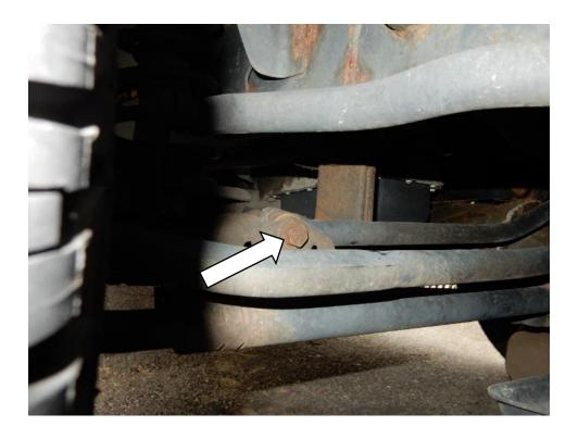
40. Using a 21mm socket and wrench, remove the bolt connecting the front track bar to the frame, remove the front track bar.
