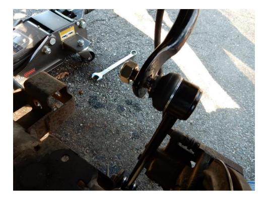
24. Position the lower bumpstop into place on the frame, aligning the mounting holes with the existing holes on the frame of the vehicle.
