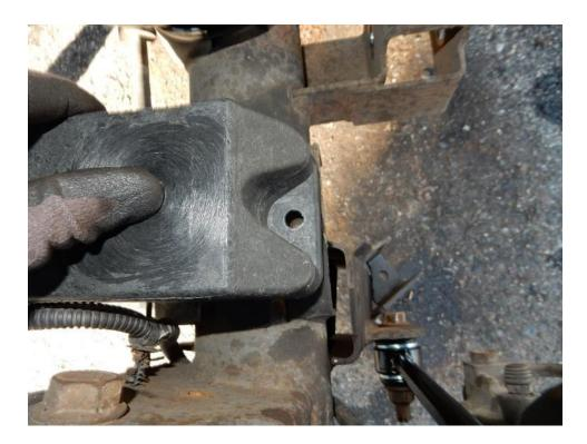
25. Using a 13mm socket and wrench, install provided bolts, nuts, and washers to attach the lower bumpstop extension to the frame on the driver and passenger sides.
