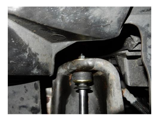
59. Using an 18mm socket and wrench, torque the lower shock bolt to 57 ft-lbs on the driver and passenger sides.
