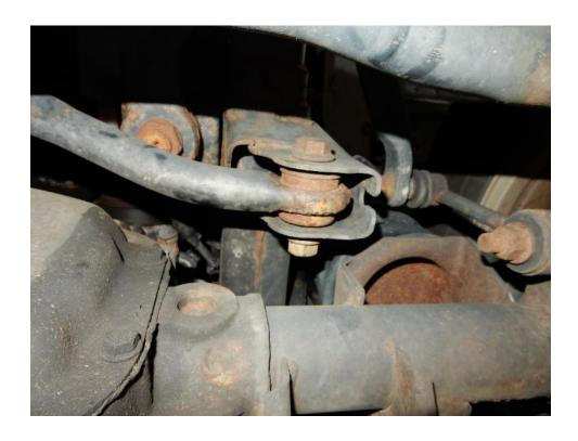
66. Position the front track bar in place at the axle mount. Using a 21mm wrench and socket, reinstall the factory bolt and nut. Torque to 125 ft-lbs.
