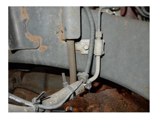
53. Using the floor jack, carefully lower the front axle far enough to remove the springs from the driver and passenger sides.
