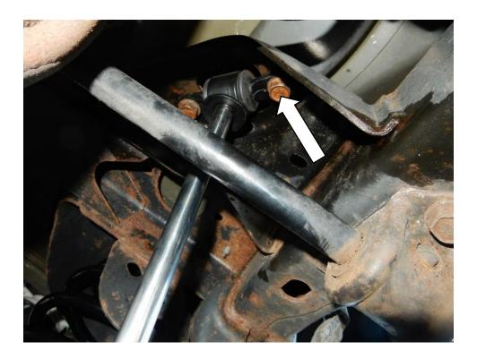
33. Position the new rear shocks in place, aligning the lower bolt holes. Using an 18mm socket and wrench, install the factory lower bolts and nuts to attach the rear shocks on the driver and passenger sides. Torque to 56 ft-lbs.
