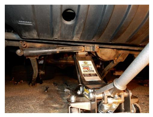
45. Place jack stands under the frame, lower the floor jack until the vehicles weight is fully supported by the jack stands.
