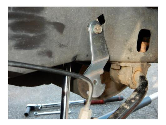
35. Using a 7/16" socket and wrench, install the supplied bolts, washers, and nuts to attach the factory brake line bracket to the brake line extension bracket on the driver and passenger sides. Torque to 120 inch-lbs.
