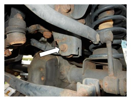
41. Using a 21mm socket, loosen the bolts on the front upper control arm on the driver and passenger sides. *Note: DO NOT REMOVE THE BOLTS OR CONTROL ARMS*
