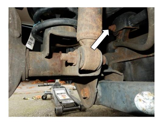
42. Using a 21mm socket, loosen the bolts on the front lower control arm on the driver and passenger sides. *Note: DO NOT REMOVE THE BOLTS OR CONTROL ARMS*
