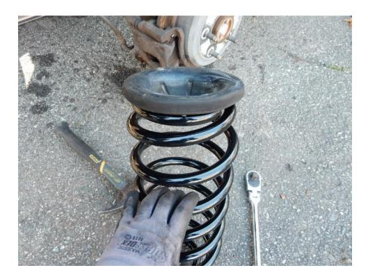
19. Install the new springs and isolators into position on the driver and passenger sides.
