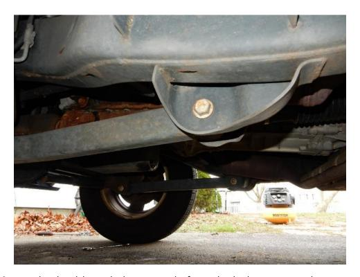
43. Using a 19mm socket, break loose the lug nuts on the front wheels, do not remove the nuts completely.
