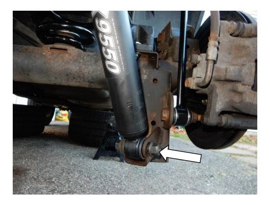
34. Position the rear brake line extension bracket in place, aligning the bolt hole with the hole in the frame where the factory bracket was attached. Using a 10mm socket, install the factory bolts to attach the bracket to the frame on the driver and passenger side.
