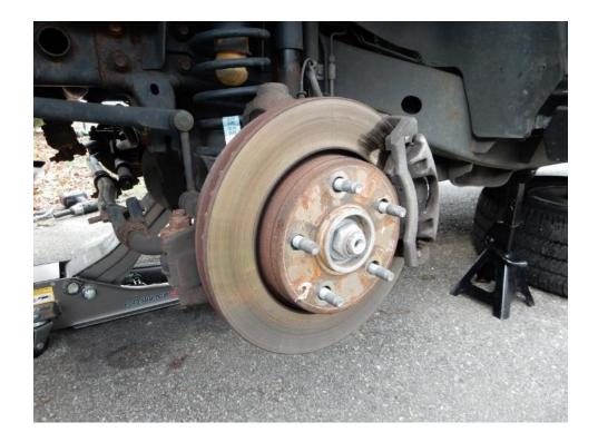
47. Using a floor jack, slightly raise the axle to make it easier to remove factory hardware.
