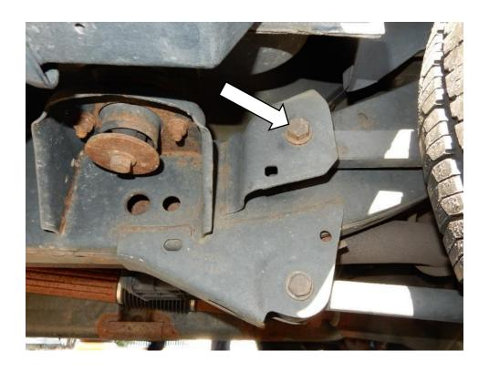
4. Using a 21mm socket, loosen the bolts on the rear lower control arm on the driver and passenger sides. Note: **DO NOT REMOVE THE BOLTS OR CONTROL ARMS**
