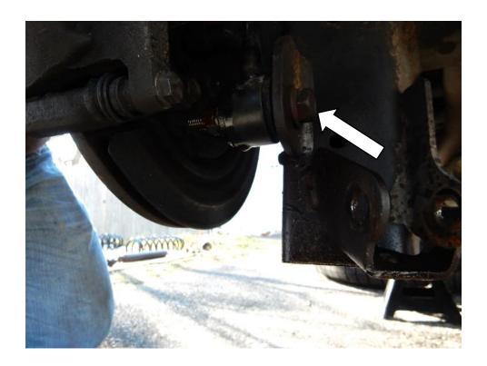
12. Using an 18mm socket, and a 19mm wrench to keep the stud opposite the nut from spinning, remove the nut from the sway bar side of the sway bar link on the driver and passenger sides. Remove sway bar links.
