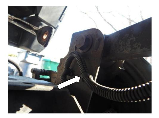
14. Using a 10mm socket, remove and discard the parking brake cable bracket from the underside of the body.
