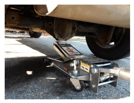
7. Place jack stands under the frame, lower the floor jack until the vehicles weight is fully supported by the jack stands.
