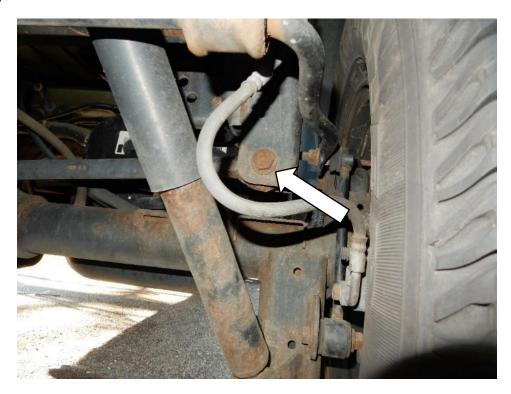
3. Using a 21mm socket, loosen the bolts on the rear upper control arm on the driver and passenger sides. Note: **DO NOT REMOVE THE BOLTS OR CONTROL ARMS**
