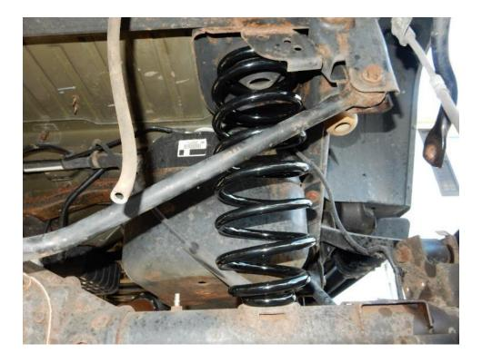
20. Using the floor jack, raise the rear axle just high enough to put pressure on the springs and hold them in place.
