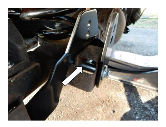
30. Position the provided U-bolt around the axle and into the bracket. Using a mm socket, attach with the provided washers and nuts. Torque to 85 ft-lbs.
