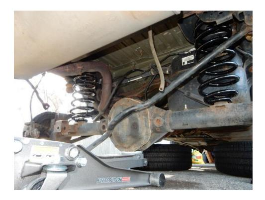
21. Install the spring retainer plates, on the driver and passenger sides, using a 14mm wrench on the bolt and the supplied wrench on the nut below the mount.
