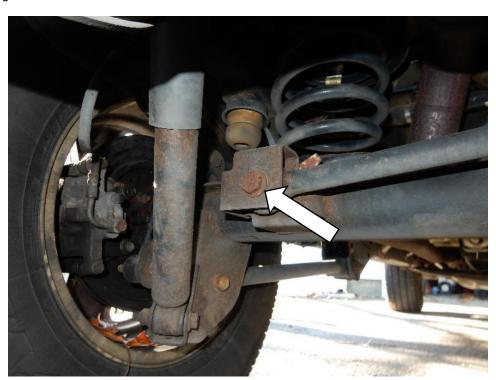
2. Using a 21mm socket and wrench, remove the bolt connecting the rear track bar to the frame, remove the rear track bar.
