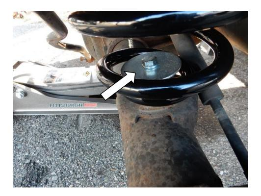
22. Using an 18mm socket and wrench, reinstall the factory bolt and nut to attach the axle side of the sway bar link to the axle bracket on the driver and passenger sides. Torque to 75 ft-lbs.
