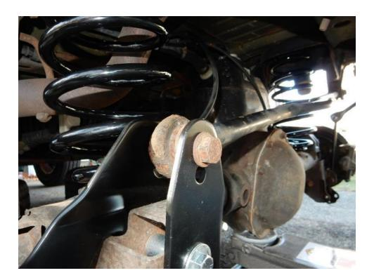
32. Position the new rear shocks in place, aligning the upper bolt holes. Using a 16mm socket, install the factory upper bolts to attach the rear shocks on the driver and passenger sides. Torque to 37 ft-lbs.
