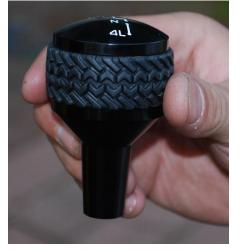
5. Remove the tire tread from the new shift knob. You should be able to pry under it with a fingernail. There is a set screw under the tire tread.
