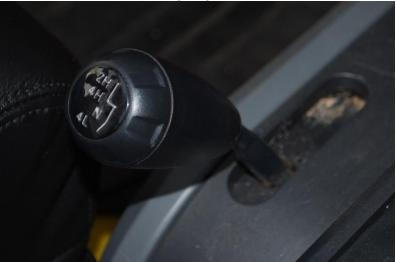
3. Pull <u>very</u> hard on the factory 4wd shift knob. The knob is fastened by a barb on the bottom of the shifter and will pull straight off. If you have eaten your Wheaties, it will pull off. If not, using the optional strap wrench, twist the knob clockwise and counter-clockwise a few times, this will help break it free from the barb.
