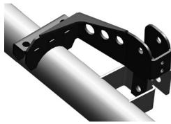
Using the supplied U-Bolt (C), 1/2" Flat Washers (D) and 1/2" Nylock Nuts (E), loosely fasten Relocation Bracket to axle tube. **Do not tighten U-Bolt nuts yet.**
