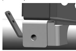
With hole in Riser Brace (B) aligned with original track bar mounting hole, insert the original track bar mounting bolt through the factory bracket, Riser Brace and mounting tab of Relocation Bracket (A).
