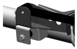
O Secure rear track bar to Relocation Bracket (A) by inserting supplied M14 x 80mm Bolt (I) through mounting hole. Bolt must be installed from the front to the rear of the vehicle.
