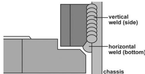
If weld bead interferes with re-installation of Pillow Block, you must remove any protrusions using a grinding wheel for proper fitment.
