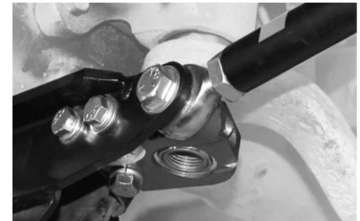
**HINT:** The extra 1/2" Locking Nut (W) & 1/2" Flat Washer (V) supplied with Front Trackbar Chassis Brace are not used when mounting to Steering Sector Pillow Block (E).
