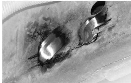
**HINT:** A die grinder with a sanding wheel is useful for removing paint from chassis.
