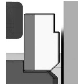
**HINT: A small gap between the weld-on mount and chassis is normal and acceptable.**
