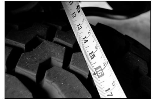
**HINT:** For example, measure from the edge of a tire tread lug to the outboard side of the chassis, then repeat the measurement on the other side of vehicle using exact same points.
