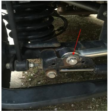
• Finally, tighten the jam-nut on the track bar.
