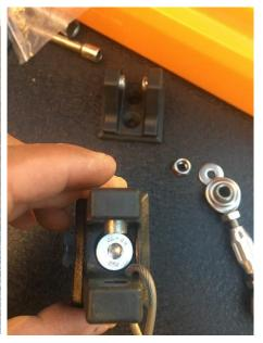
• Install on the fender where the old latch was removed using a M8 nut and washer. It's easiest to use the allen wrench for most of the tightening as there's limited room to swing the ratchet. Be careful to not overtighten.
