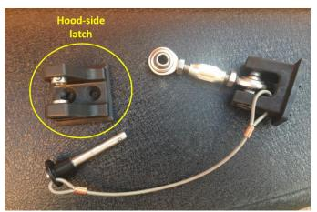
Place a square rubber pad on the bottom of the hood-side latch and use two M6 hardware sets (allen bolt, washer, and Nyloc nut) to mount the latch to the old one's location. Note that the M6 washers have a larger outside diameter than the M8 ones.
