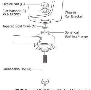
**HINT**: Tapered Split Cone (N) should be located between flange of spherical bushing (L) and mounting surface of chassis rail bracket, with the narrow end of tapered cone facing <u>up</u> towards chassis.
