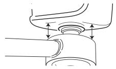
IMPORTANT: The Chassis End of Adjustable Trackbar must be in the "neutral" position (as illustrated above) <u>before</u> the Jam Nut is tightened.
