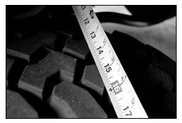
**HINT**: For example, measure from the edge of a tire tread lug to the outboard side of the chassis, then repeat the measurement on the other side of vehicle using the <u>exact</u> same points.
