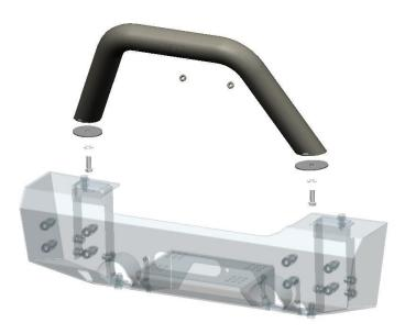
1. Loosely Place the two **Gaskets** between the **Light Bar** and the top face of the bumper.
