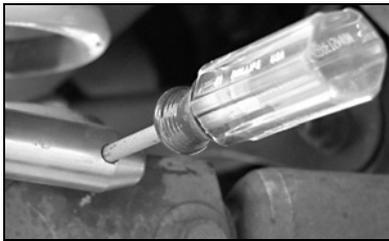
**HINT:** A small Philips head screwdriver or punch inserted into the Click Pin hole will enable you to prevent the Stainless Steel Post from rotating when tightening the mounting bolt.
