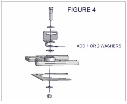
• If the key cannot be removed when the box is locked. The lock may not be centered in the mounting hole. With the key removed in the unlocked position, while looking at the lock-cam from under the lid, lightly push the cam counterclockwise until it stops. This will slightly rotate the camlock in the mounting hole.
