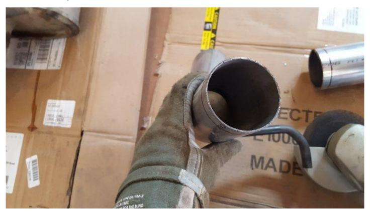
**13.** Insert the over axle pipe into the rear of the muffler as shown with the metal hanger facing the rubber hanger and with the clamp in place loosely. Make sure it is fully inserted into the muffler and is angled up over the axel.
