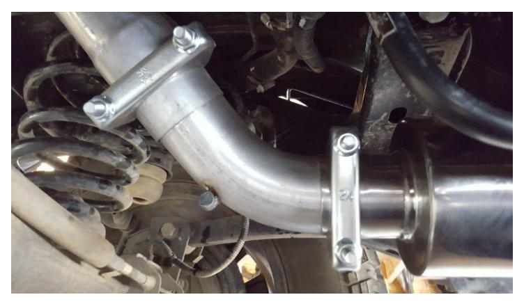
**14.** Next place the tail pipe over the axle as shown below. Place on the clamp and attach it to the over axle pipe as shown above. Attach the rubber hanger shown by the arrow below to hold the tailpipe in place.
