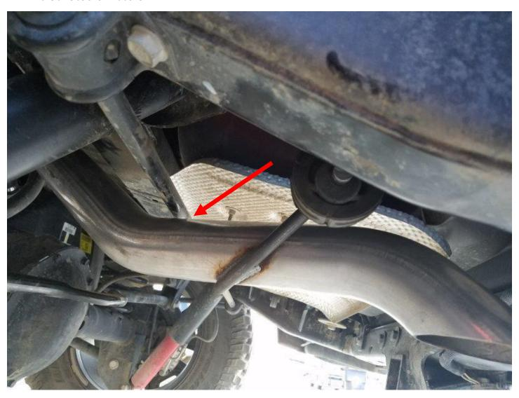
**16.** When all the pipes are aligned properly you can tighten all the clamps using a 14mm socket. I recommend turning the clamps to the side to maximize you're clearance. You will need to make these clamps pretty tight to ensure a good seal at each joint.
