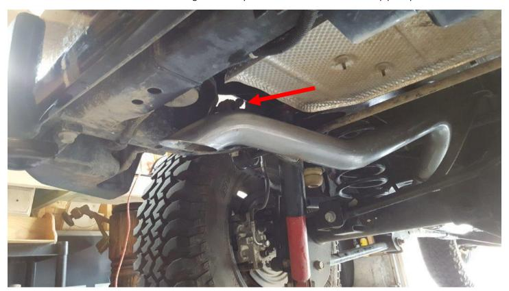
**15.** Before tightening any of the clamps you will need to adjust the exhaust pipes for proper positioning. Make sure all pipes are not touching any other parts. As shown below, the exhaust pipe can come close to the rear sway bar. You can give it a little more clearance from the sway bar by angling the over axle bend as shown above.
