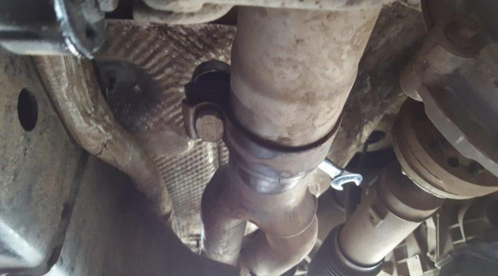
2. Next remove the transfer case skid plate located below the driver door. It is possible to complete the install without removing it, but it will be much easier if removed. You will need to remove the four 18mm bolts holding the skid plate on.
