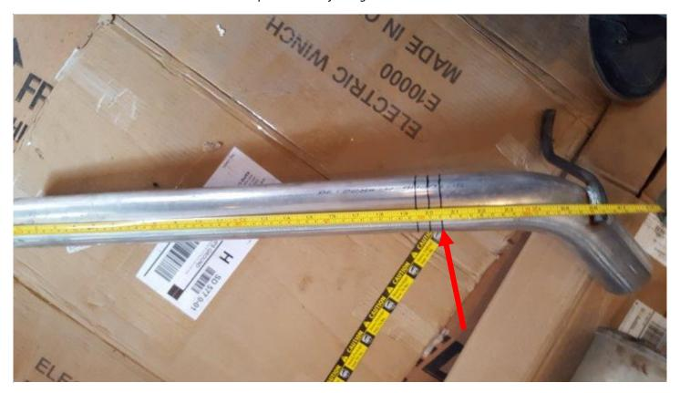
11. Using an angle grinder, cut the pipe along the line you marked. Make sure to wear gloves and safety glasses.
