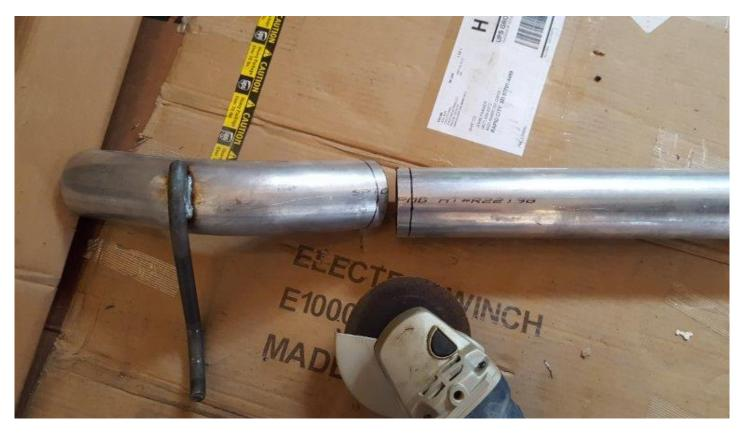
**12.** Make sure to clean up the cut as shown below. Metal left outside will make it difficult to install, and metal left inside will impede exhaust flow.
