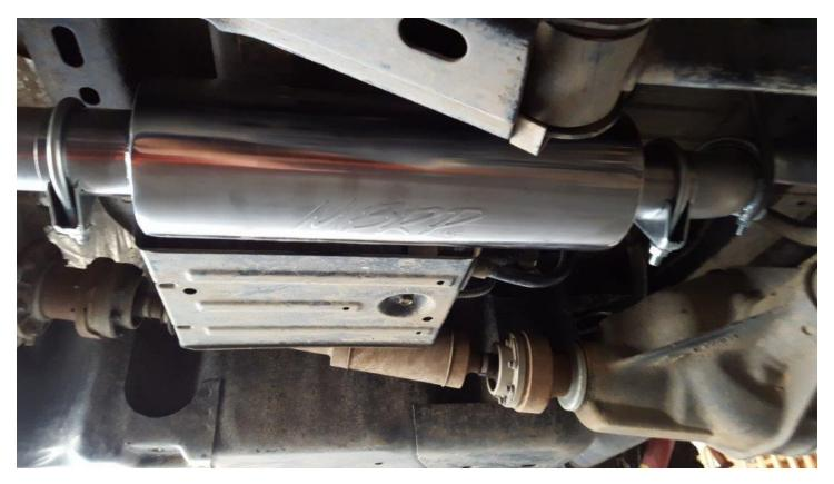
10. Steps 10-12 are only required for 2dr installation. Using a tape measure and sharpie, measure and mark 20 ½" on the over axle pipe. Make multiple marks around the pipe and draw the line all the way around. Note:
