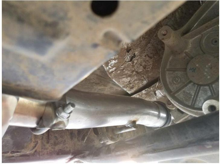
**9.** Now attach the muffler to the short extension pipe. Make sure to put the clamp in place before putting the muffler on. The muffler can face either direction, so put it however you think looks best. I chose to have the MBRP label showing.
