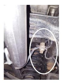
12. Slide the final  $2\frac{1}{2}$ " clamp and install the tail pipe (included with your kit) on the "over the axle pipe." Attach the tail pipe to your factory rubber insulator.
