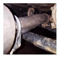
**9.** Slide a second 2  $\frac{1}{2}$ " clamp over the extension pipe and install the new MBRP muffler. Remember don't tighten any clamps till final adjustment.
