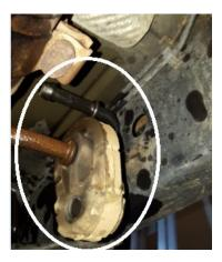
7. Remove the hanger from the existing rubber insulator right before the rear axle.
