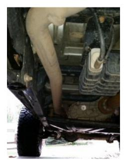
**1.** Loosen the transfer case guard and remove using the 3/4 inch socket. One bolt on the frame side and another at the gas tank.
