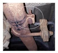
**6.** Remove the hanger from the existing rubber insulator on the extension pipe.
