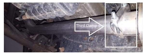
11. Attach the "over the axle pipe" to the factory rubber insulator.
