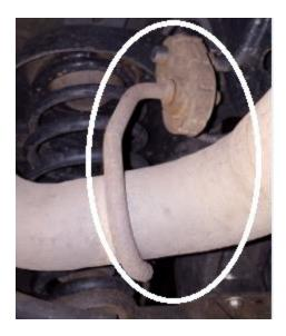
This picture shows the hanger removed from the rubber insulator.
