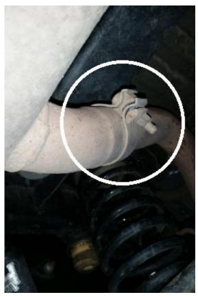
**3.** Then remove the hangers from the rubber insulator, one on each side. This is the passenger side by the frame.
