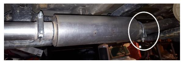
**10.** Install the third  $2\frac{1}{2}$ " clamp over the new muffler and slide on the "over the axle pipe" to the muffler.
