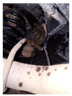
**8.** You can now start installing your new MBRP exhaust system, start the install by using one of the four 2 1/2" clamp that's provided. Than attach the new extension pipe to the existing rubber insulator and leave the clamp loose until final adjustment.
