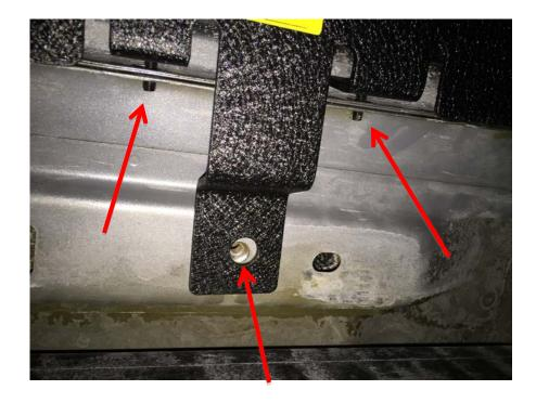
**Step Six:** Now proceed to tighten all of the bolts and nuts completely using the 10mm socket wrench with  $\frac{1}{2}$ " rachet for the hex bolts and the 13mm socket wrench with  $\frac{3}{8}$ " rachet for the lock nuts.
