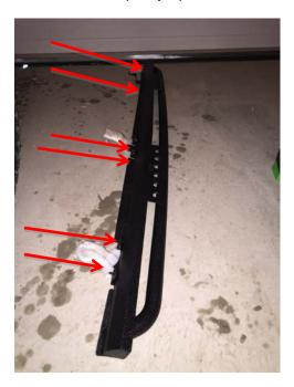
**Step Five:** Insert  $3 - 8 \times 35$ mm hex bolt with 8mm flat washer into the pre-threaded holes from the factory and 6 - 6mm Ny-lock Nut with 6 - 6mm flat washers onto the bracket study that go through the pinch weld.
