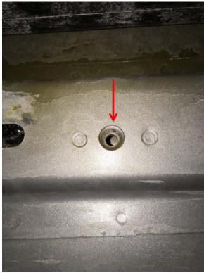
**Step Four:** Take the driver side rock rail/step and loosely attach it to the jeep by lining up the 6 tabs on the rock rails with the already existing holes on the pinch weld area on your jeep.
