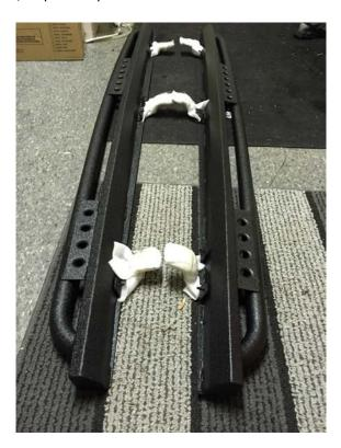
**Step Three:** Identify the 6 existing holes in the pinch weld (2 front, 2 center, 2 back) and the 3 pre-threaded holes that come from the factory\*\*\*
