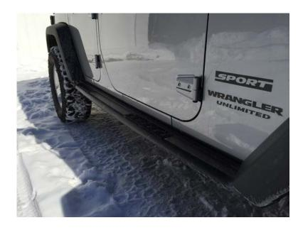
\*\*\*Note: As stated in Step Three my jeep has pre-threaded holes from the factory, on some 2012 and older models you will use the nut-clip setup provided by Smittybilt with 10mm bolts. There will be an open cavity area in the bottom of the body tub. You will install the nut-clips the same way the 8mm bolts were installed
