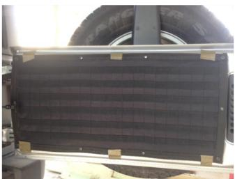
2. Once secured, begin drilling the screw holes using a 7/64" drill bit. As you install the included screws make sure to pull all of the slack on the cover to avoid sagging, and do not over tighten the screws. Note: On 2011 models and up, you will need to drill two extra holes for the tailgate support bracket.
