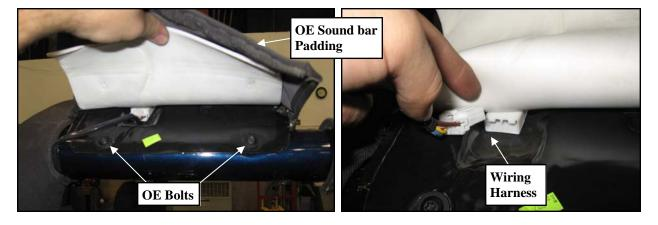
**Step 6:** Pull the padding to one side of the side support bars to reveal the **OE** sound bar bolts and wiring harness. Unclip the wiring harness.
