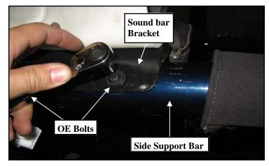
**Step 7:** Remove the **(2 per side) OE** bolts connecting the **OE** side support bars to the soundbar bracket.
