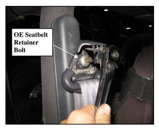
**Step 4:** Unbolt and remove the shoulder strap adjuster mounts from the vehicle. Save hardware for reinstallation.
