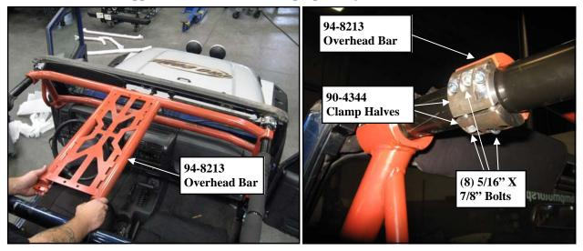
**Step 10:** Install the main support cage mounts to the **OE** cage main support hoop . (94-4408).
