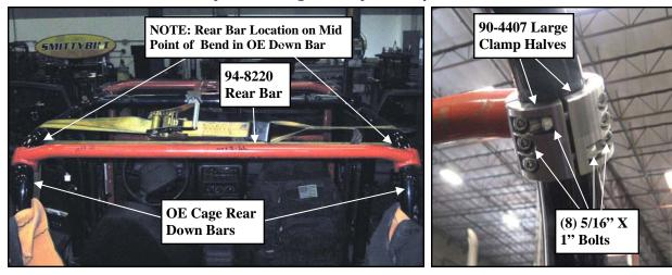
Step 13: Install the rear cross bars (94-8216 Drvr and 94-8218 Pass) to the OE main cage. Secure to the OE rear down bars using the (90-4407) large clamp halves, and (8 per side) 5/16" X 1" bolts. Secure the main cage support mounts using the (2 per side) supplied 5/16" X 1 1/4" bolts. NOTE: They will need to be slid in from the center out.
