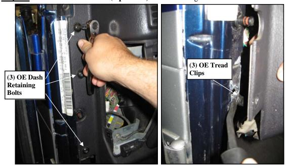
**Step 19:** Carefully, pull the dashboard back far enough to access the (**3 per side**) tread clips. Remove all the tread clips and push the dashboard back.
