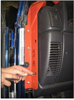
**Step 25:** Reinstall the previously removed front shoulder strap adjuster mounts using the previously removed **OE** hardware.
