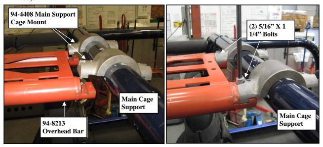
Step 11: Slide the overhead bar (94-8213) back and interlock the clamps with the Main Support cage mounts (94-4408). Secure using the (2 per side) supplied 5/16" x 1 1/4" bolts.
