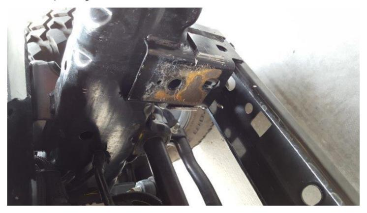
**12.** Use a wire brush or sandpaper to remove any rust that was under the bracket.
