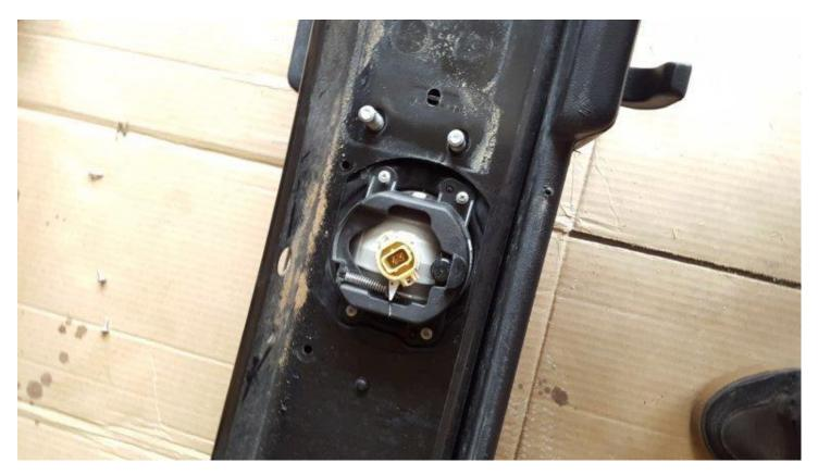
17. I had to drill out the holes to make them a little larger so they would fit in the new bumper. Use the 3/16" drill bit and drill out the holes.
