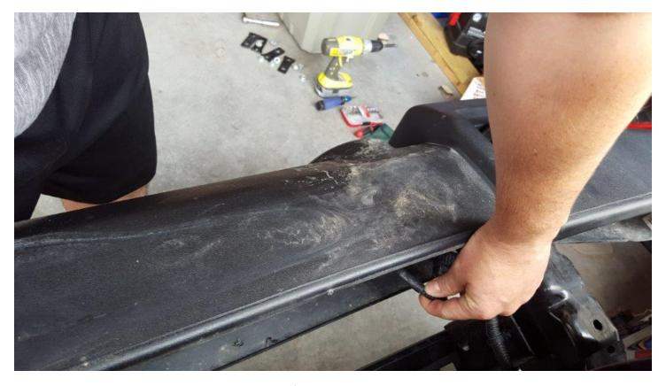
**6.** Remove the plastic retainers that attach the fog light wires to the bumper.
