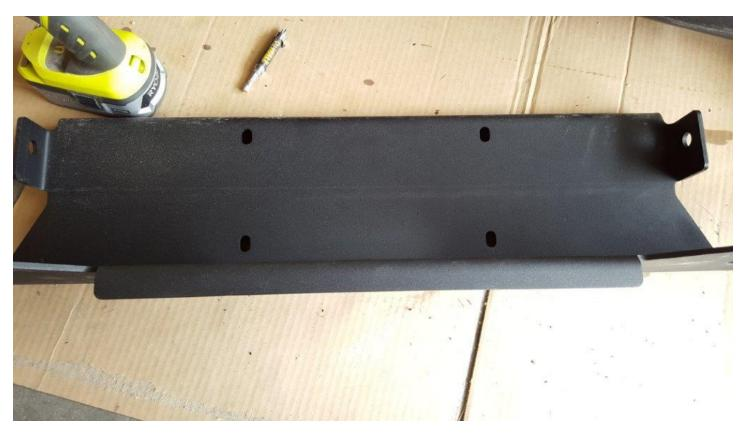
**29.** Now you are ready to install the winch plate. I highly recommend having someone hold the winch/winch plate in place while you insert the bolts. Slide the winch plate in between the frame rails as shown in the next 2 pics. Insert the two ½"x1½" bolts and washers shown. If you used the canister relocation bracket, make sure the winch plate is between the bracket and the frame as shown below.
