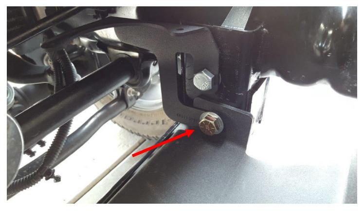
**33.** Using the supplied bolts, install the canister onto the new relocation bracket. I recommend using washers also (Not supplied).
