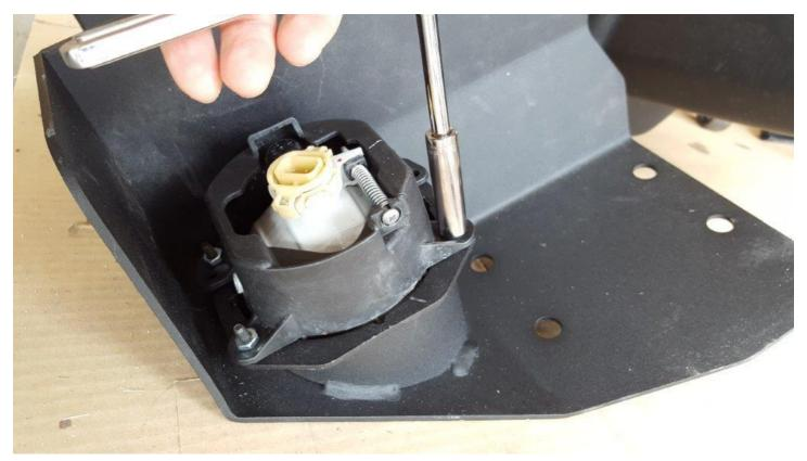
**20.** Unfortunately the stock fog light wires are not long enough to reach both fog lights once the bumper is installed. You will need to splice in roughly 10-12" of wire to each fog light connector. Start by stripping the tape and plastic tubing from the wire. Then cut the wires as shown.
