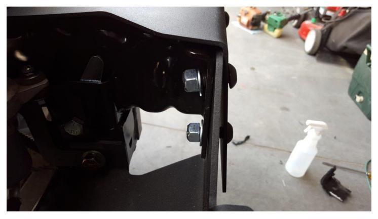
**35.** Rough country says the allen bolts are 8mm, but I found that 5/16" allen bit worked better. You can use either. Using the allen bit and 3/4" deep well socket, fully tighten all 8 bolts on the front of the bumper.
