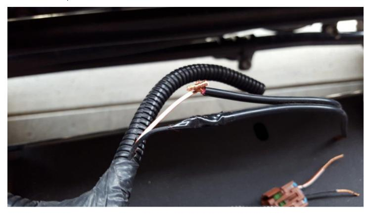
**24.** Then connect the wiring harness that was cut off (shown above on the bottom right) twist and tape the wires in the same fashion. Make sure the wires still match up to the correct color wires.
