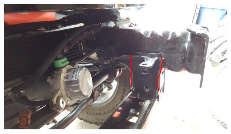
**11.** Once you have removed the bracket it should look about like this. I recommend using the grinder to smooth out the sharp metal edges.
