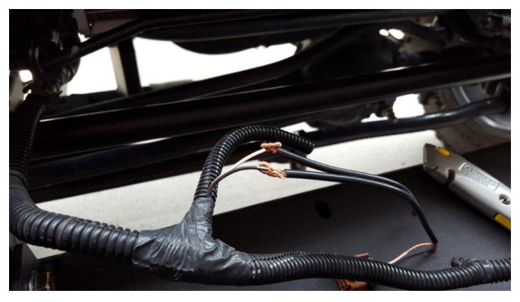
**23.** Tape each wire individually, then tape them together. Make sure the tape overlaps at least an inch on either side of the splice.
