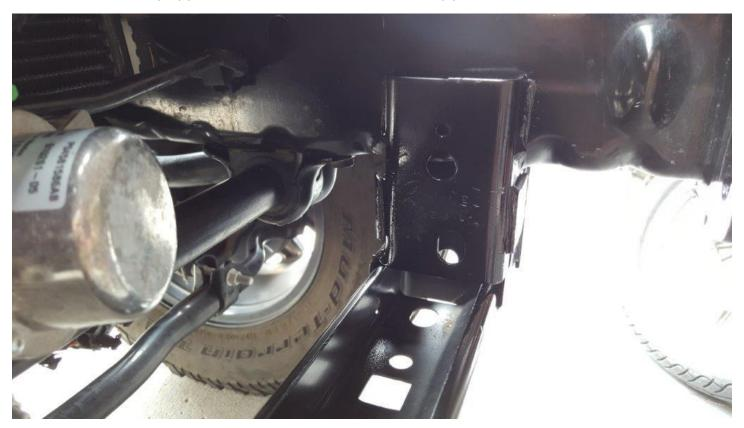
**14.** Place the ½" x ¾" bolt into the bracket then place the washer on the bolt so that it will be between the bracket and the frame.
