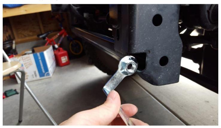
**32.** Align the flag nut installed above with the bolt installed in step 29. Tighten the bolt using a ¾" socket. Do not fully tighten until you have installed the end caps and front bolts.
