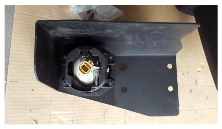
**19.** Using the supplied nuts and a 10mm deep well socket tighten the 4 nuts on both fog lights. Be careful not to overtighten or you could break the bracket.
