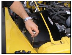
**14.** Using the supplied ½ x 20 nut, bolt and washers, mount the front of the Airaid Cool Air Dam to the inner fender.
