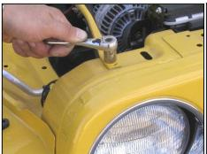
**9.** Using a 13mm socket, remove the radiator rod support bolt on the passenger side. Retain bolt for later use.
