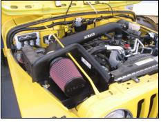
**28.** Install the weather strip on the edge of the Cool Air Dam assembly as shown above. Reconnect negative battery cable. Double-check your work to be certain that all nuts, bolts, and clamps are securely fastened.
