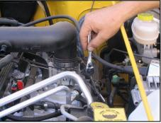
**2.** Loosen hose clamps on both ends of factory intake tube. Remove intake tube from engine.
