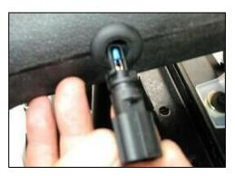
**3.** 2005-06 Vehicles: Disconnect the electrical connector to the air temp sensor on the backside of the factory intake tube and remove sensor. Retain sensor for later use.
