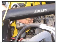
**23.** Mount the Airaid intake tube to the valve cover bracket using the supplied <sup>1</sup>/<sub>4</sub>" bolt and washer as shown above.
