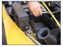
**5.** Using a 5/16" socket, remove the three nuts and bolts mounting the factory air filter housing to inner fender. Remove air filter housing.
