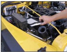
**4.** Remove factory air filter from airbox.
