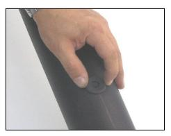
17. <u>For 1997-2004 Vehicles Only:</u> Install the supplied rubber grommet with out the hole into the Airaid intake tube.
