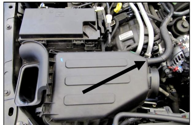
3. Disconnect the crankcase breather line in the top of the airbox. Remove the entire airbox as an assembly by unseating it from the mounting grommets in the inner fender and lifting upward.
