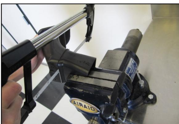
8. Firmly place the air scoop into a bench vice and cut along the line created in step 7 using a hack saw or equivalent.
