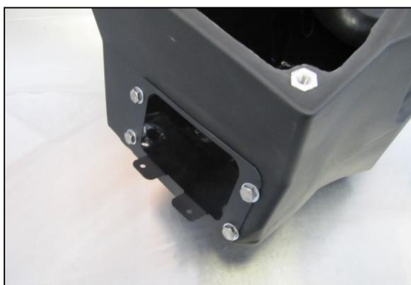
5. Install the Air Scoop Bracket (#9) into the Cold Air Box as shown by using four 1/4-20 x 5/8 Hex Bolts (#17), 1/4" Flat Washers (#11), and 1/4" Nylock Nuts (#16).
