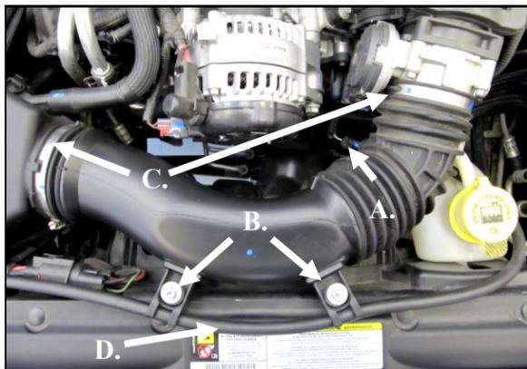
2. **A.)** Disconnect the air temp sensor in the factory intake. **B.)** Remove the two 6 mm bolts holding the intake tube to the fan Shroud. **C.)** Loosen the Clamps on both sides of the factory intake tube. **D.)** Unclip the coolant line from the intake tube and remove it from the vehicle.
