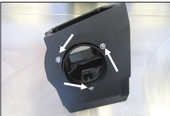
4. Install The Filter Adapter (#5) in the Cold Air Box (#3) using three 1/4-20 x 1/2" Button Head Bolts (#18) and 1/4" Flat Washers (#11).
