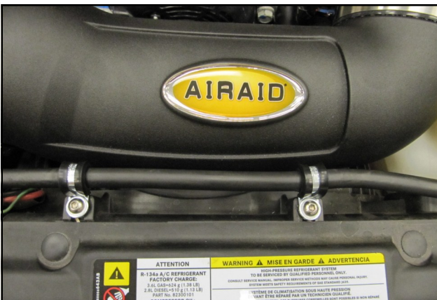
16. Secure the coolant line to the fan shroud using the two Adel Clamps (#25), 6 mm Bolts (#12), and 1/4" Flat Washers (#11).
