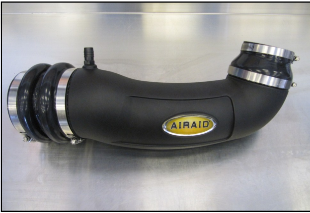
13. Slide the Double Hump Hose (#6), and two #72 Hose Clamps (#28), onto straight end of the Tube. Slide the Silicone Reducer (#7) and the #48 and #64 Clamps on the 90 deg. bend of the Intake tube. Leave the Clamps loose for now.
