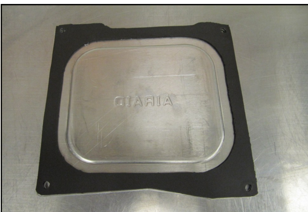
19. Place the Gasket (#8) onto the underside of the Air Box Lid (#4) and peel off the protective film. Mount the lid on the Air Box using four 1/4-20 x 1/2" Button Head Bolts (#18), and 1/4" Flat washers (#11).
